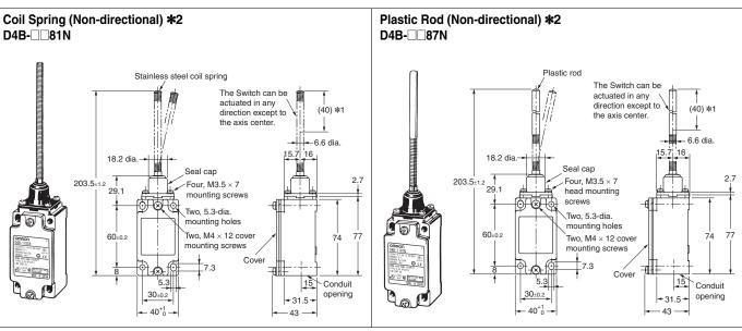
Note: Unless otherwise specified, a tolerance of  $\pm 0.4$  mm applies to all dimensions.
