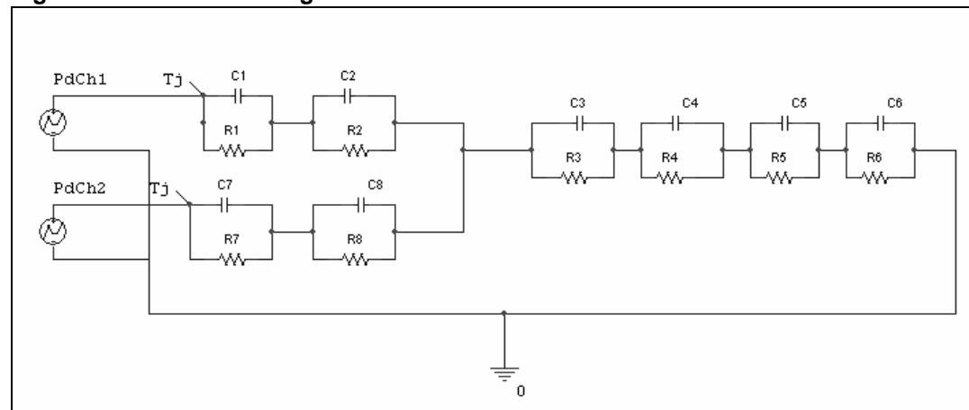
1. The fitting model is a simplified thermal tool and is valid for transient evolutions where the embedded protections (power limitation or thermal cycling during thermal shutdown) are not triggered.
