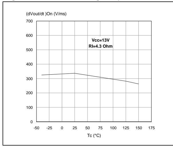
**Figure 28. Turn-off voltage slope**
