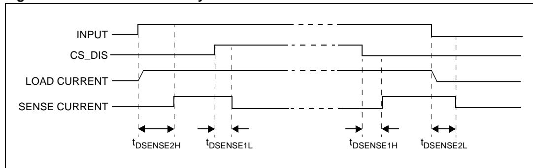
**Figure 5. Openload off-state delay timing**
