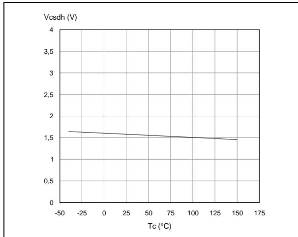
**Figure 30. CS\_DIS low level voltage**
