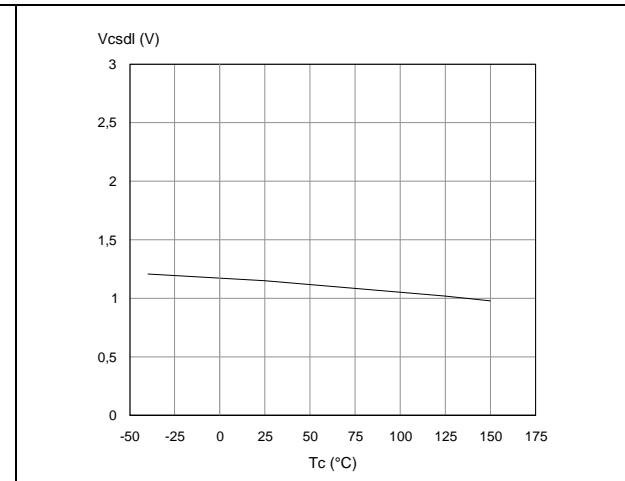
**Figure 31. CS\_DIS clamp voltage**
