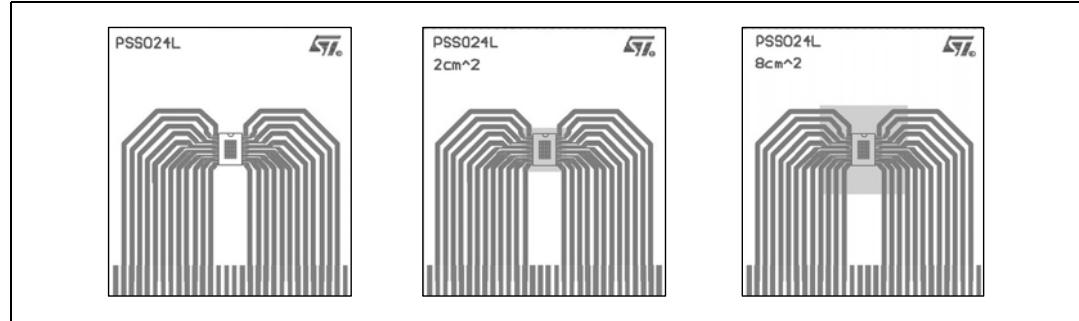
1. Layout condition of  $R_{th}$  and  $Z_{th}$  measurements (PCB: Double layer, Thermal Vias, FR4 area = 77 mm x 86mm, PCB thickness = 1.6 mm, Cu thickness = 70  $\mu$ m (front and back side), Copper areas: from minimum pad layout to 8  $\text{cm}^2$ ).
