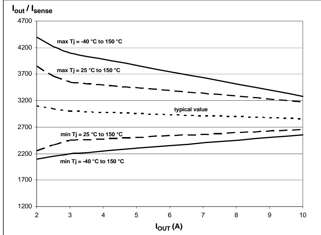
**Figure 10.** Maximum current sense ratio drift vs load current
