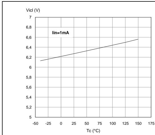
Figure 20. Input high level voltage
