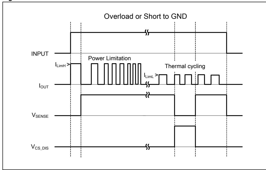
**Figure 13. Intermittent overload**
