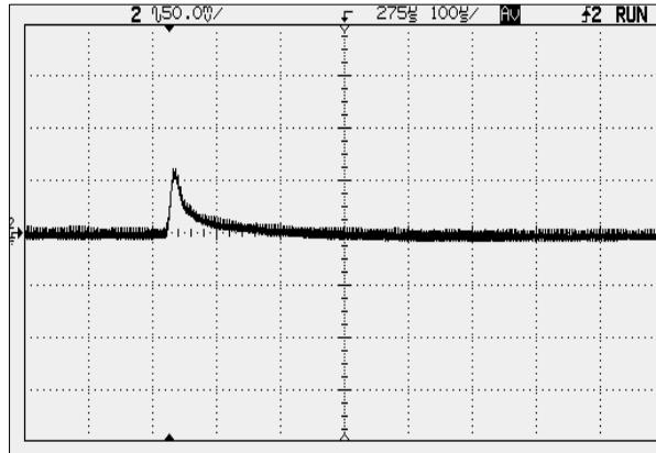
**Input Reflected Ripple (Vin=48V, Iout=50A, 2mA/div., 100uS & 10uS/div.)**
