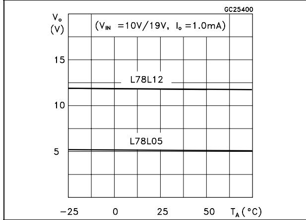
**Figure 5.** L78L05/12/24 load characteristics
