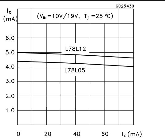
**Figure 8.** L78L05 quiescent current vs input voltage
