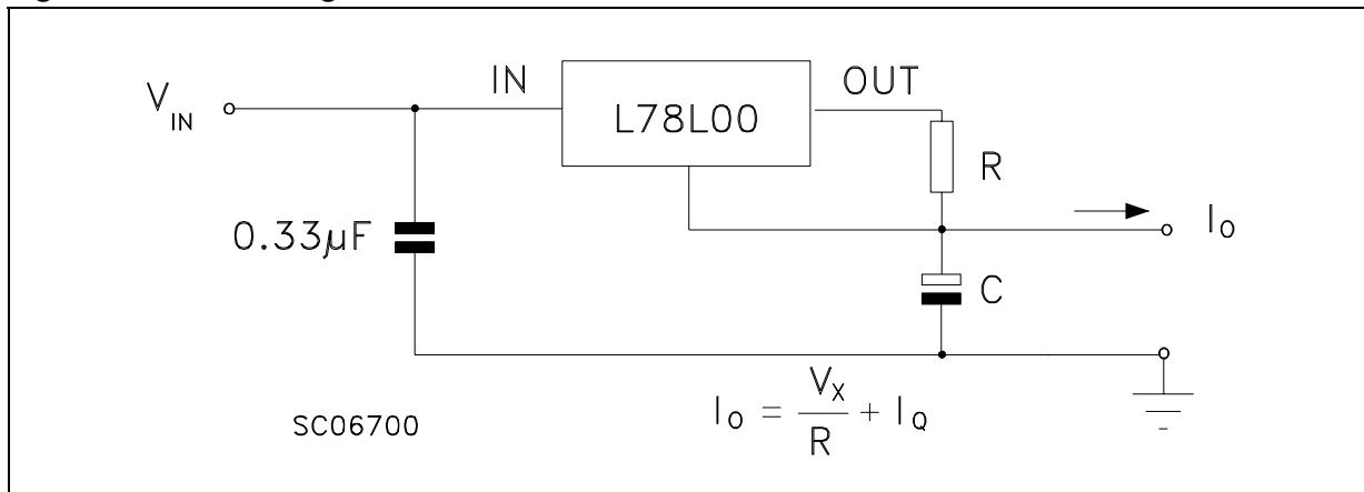
**Figure 16. Adjustable output regulator**
