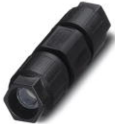
QUICKON cable connector, black, 3+PE-pos., 0.75 mm 2 ... 1.5 mm 2 / 500 V/15 A, for a cable diameter of 6 mm ... 12 mm.
