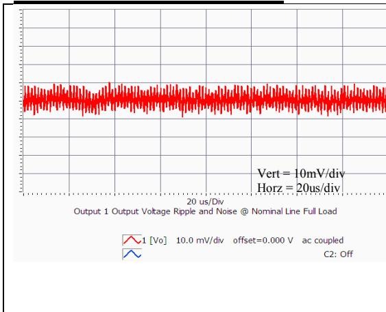
Vo=1.8V Typical Output Ripple at nominal Input voltage and full load at Ta=25 degrees
