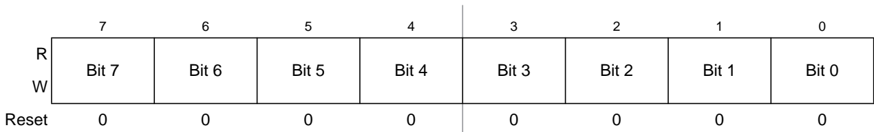
Figure 16-23. Timer Input Capture/Output Compare Register x Low (TCxL)
