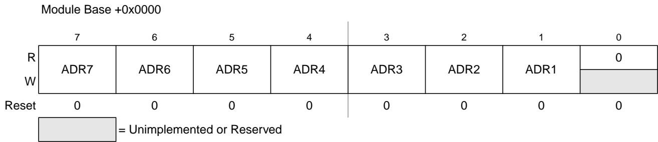
Figure 12-3. IIC Bus Address Register (IBAD)
