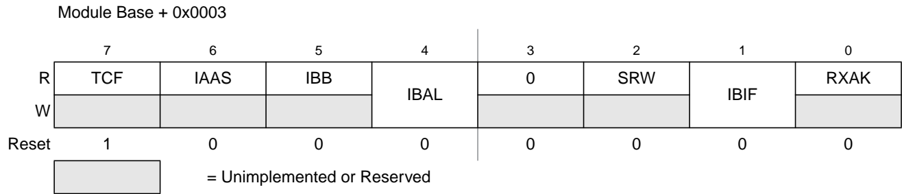
Figure 12-7. IIC Bus Status Register (IBSR)
