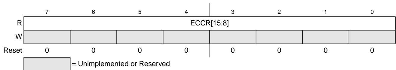
Figure 18-20. Flash ECC Error Results High Register (FECCRHI)
