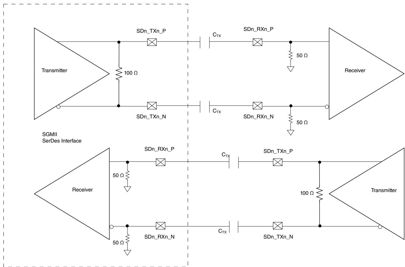
**Figure 39. 4-wire AC-coupled SGMII serial link connection example**
