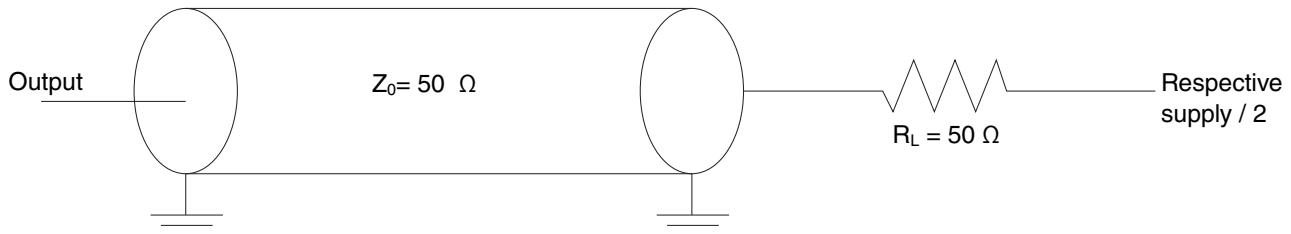
**Figure 78. AC test load for the JTAG interface**
