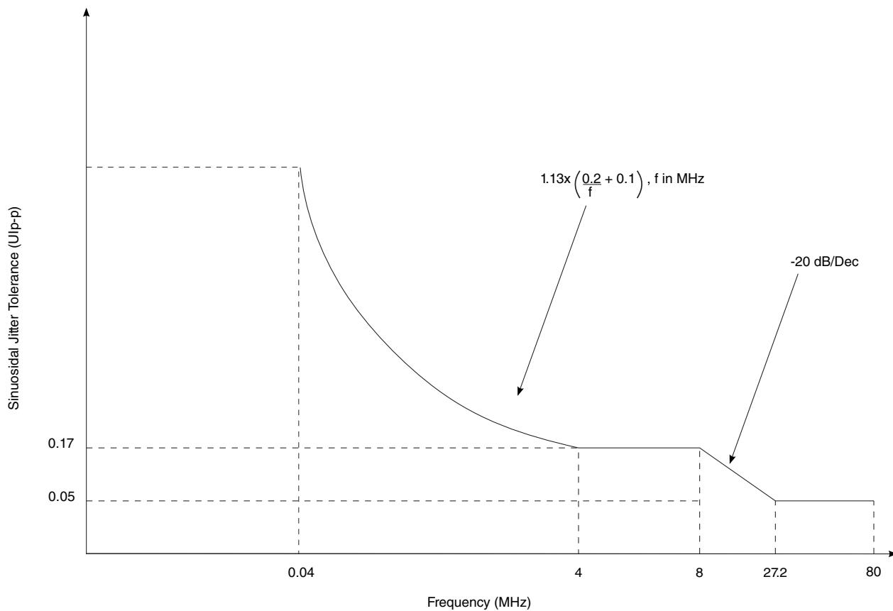
**Figure 44. XFI host receiver input sinusoidal jitter tolerance**
