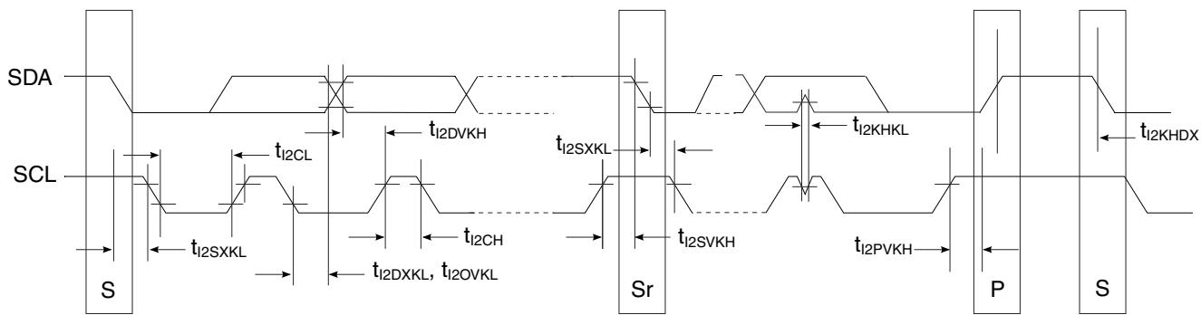
Figure 46. I<sup>2</sup>C bus AC timing diagram
