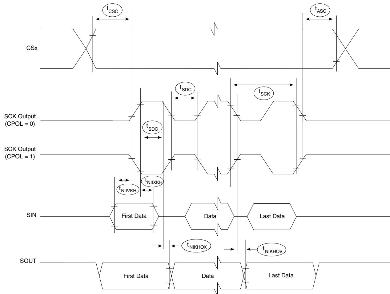
**Figure 92. SPI timing master, CPHA = 0**
