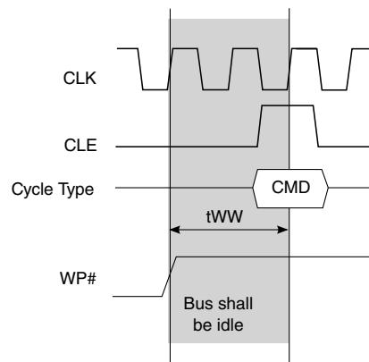
**Figure 66.  $t_{WW}$  timings**
