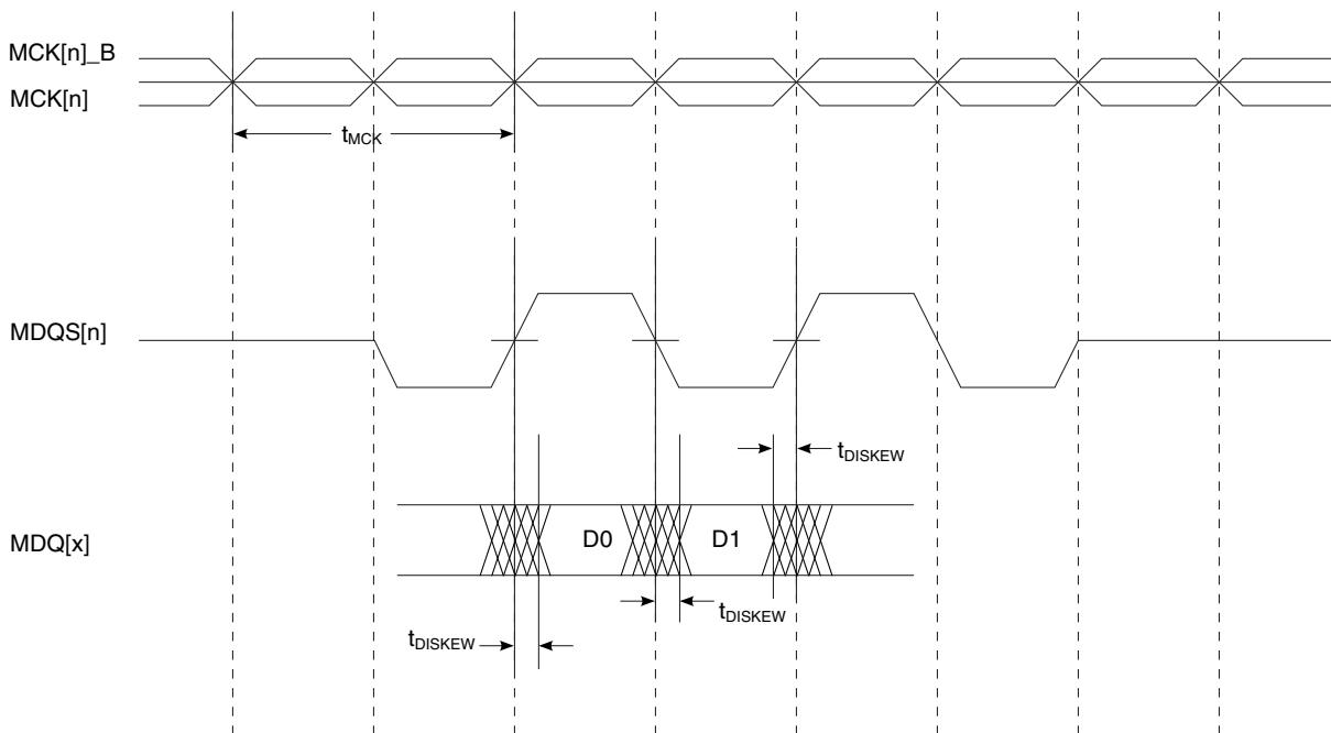
**Figure 11. DDR4 SDRAM interface input timing diagram**
