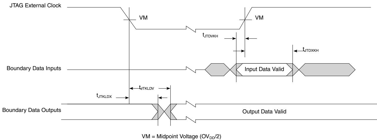
**Figure 81. Boundary-scan timing diagram**
