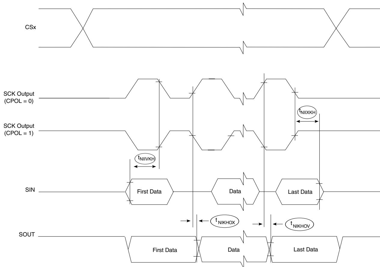
Figure 93. SPI timing master, CPHA = 1
