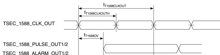
**Note:** The output delay is counted starting at the rising edge if  $t_{1588CLKOUT}$  is non-inverting. Otherwise, it is counted starting at the falling edge.
