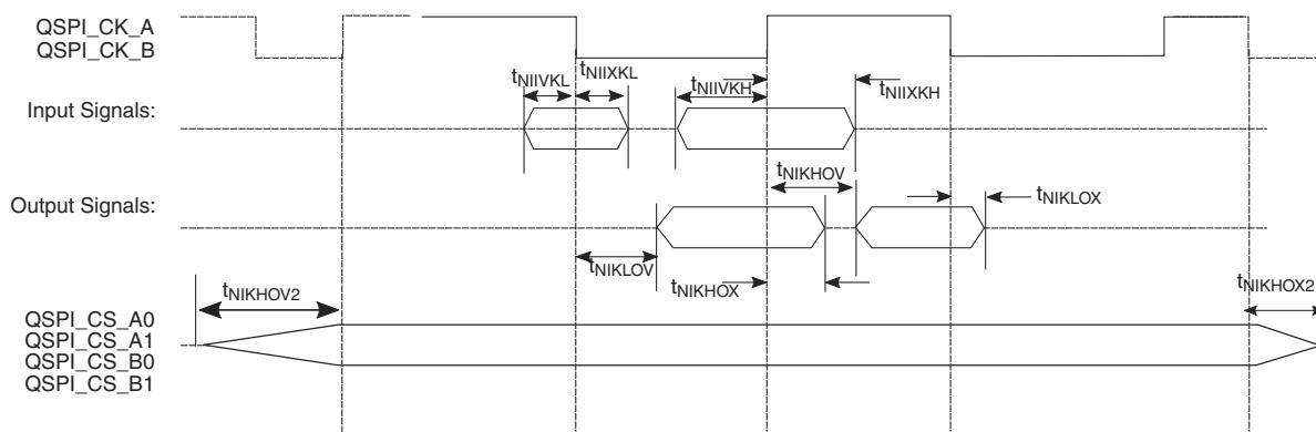
**Figure 83. QuadSPI AC timing — DDR mode**
