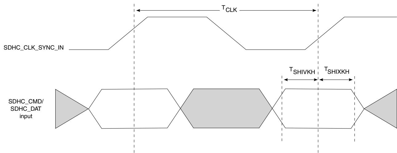
**Figure 18. eSDHC SDR50 mode input AC timing diagram**
