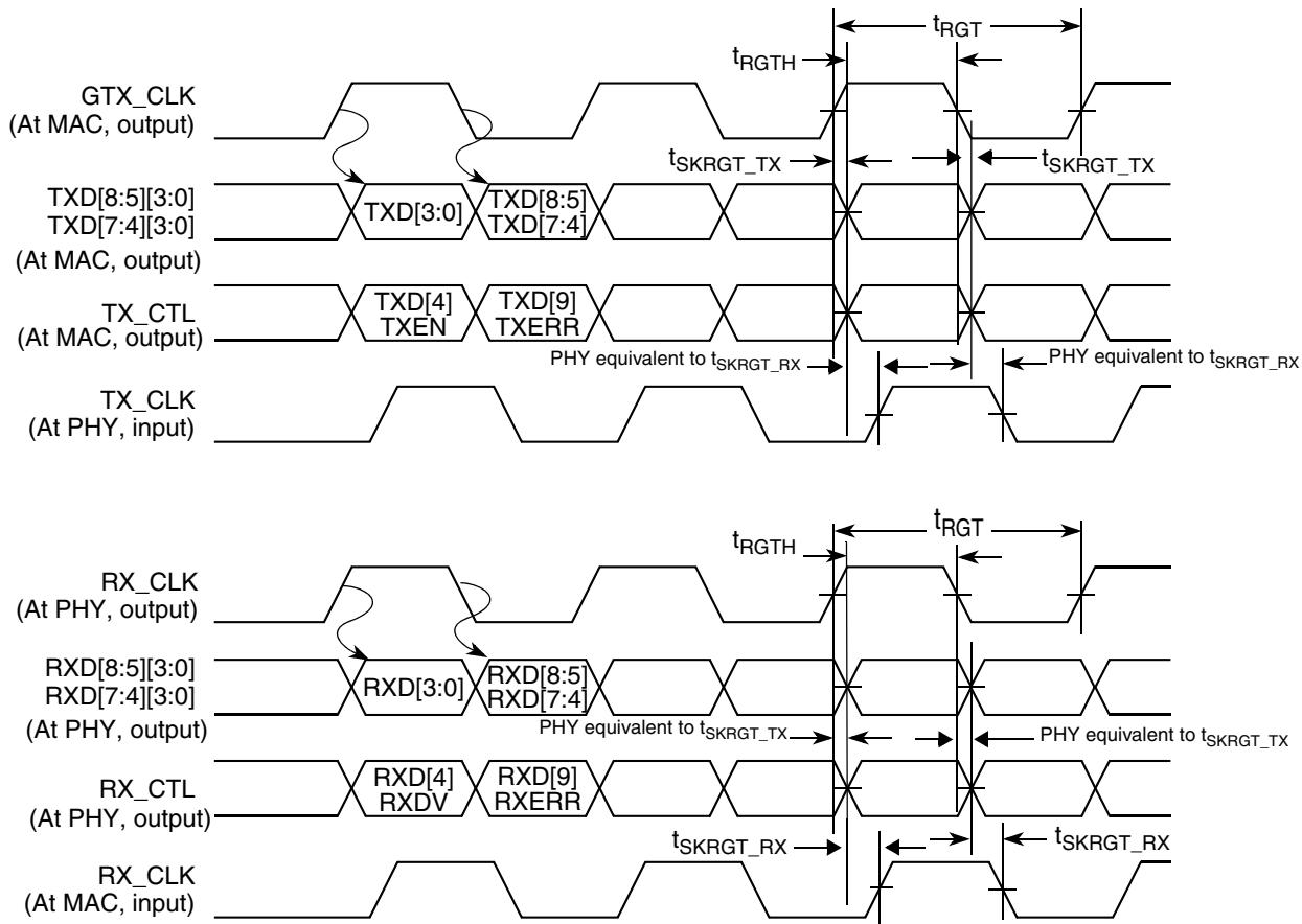
**Figure 27. RGMII AC timing and multiplexing diagrams**
