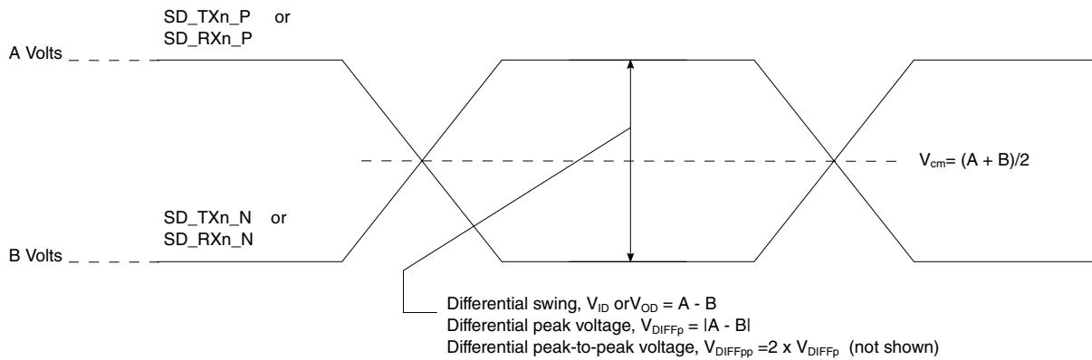
**Figure 29. Differential voltage definitions for transmitter or receiver**
