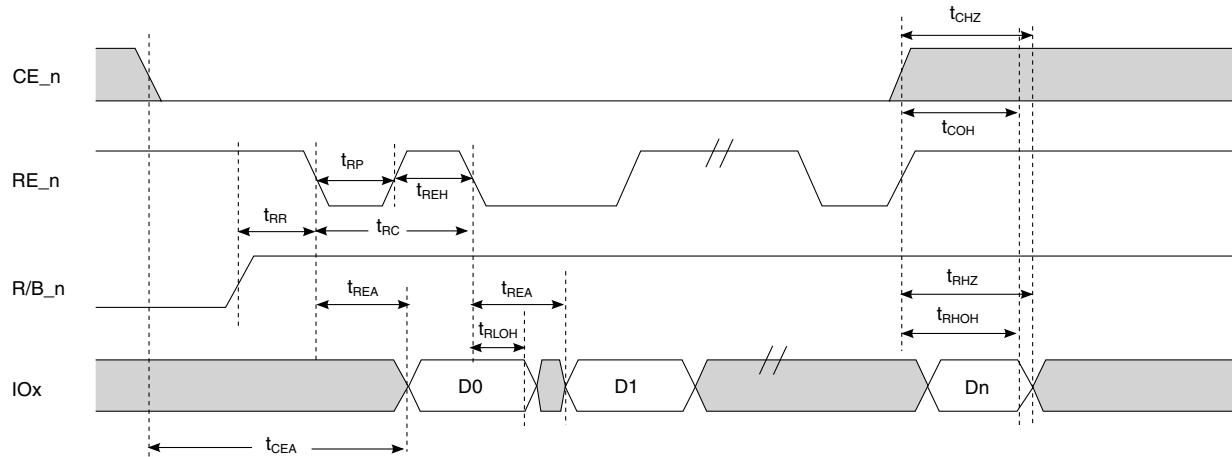
**Figure 62. EDO mode data input cycle timings**
