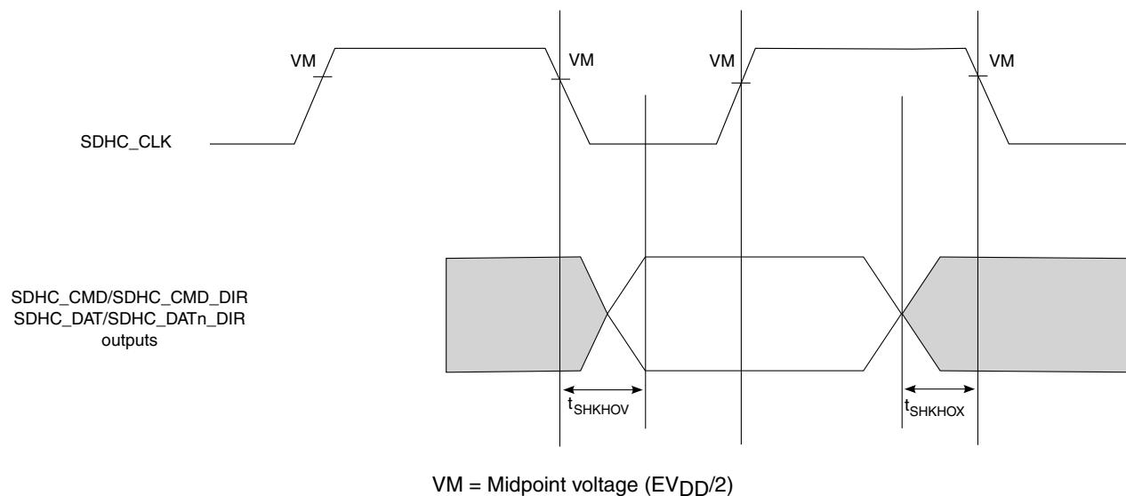
**Figure 16. eSDHC high-speed mode output AC timing diagram**
