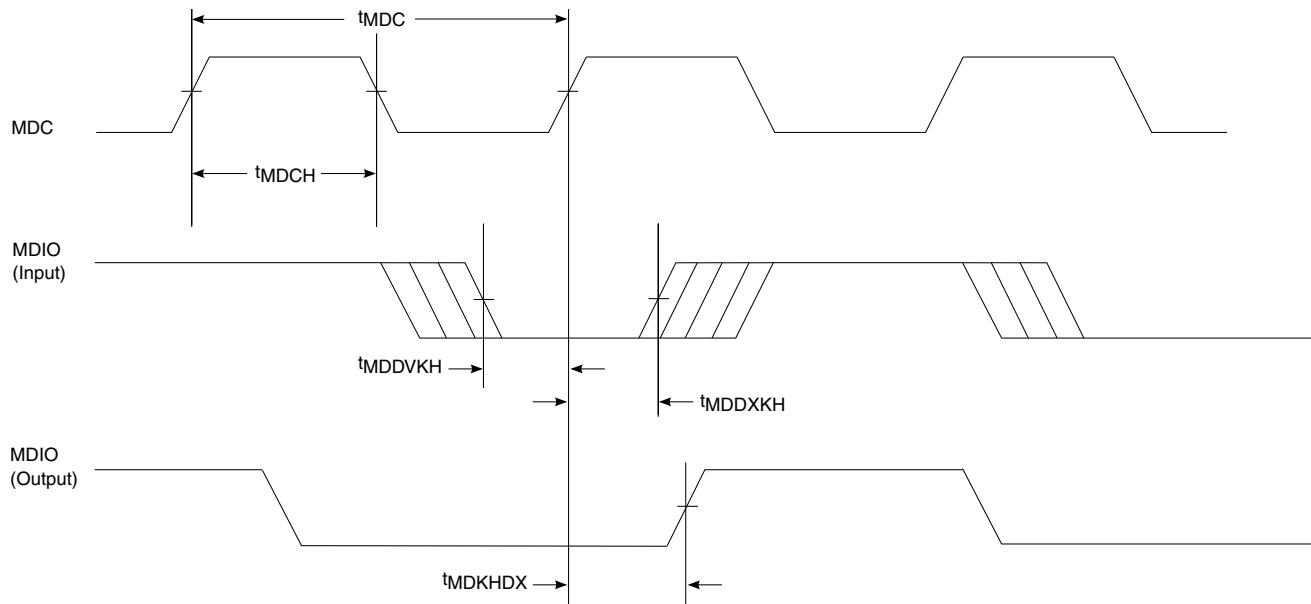
**Figure 23. Ethernet management interface 1 timing diagram**
