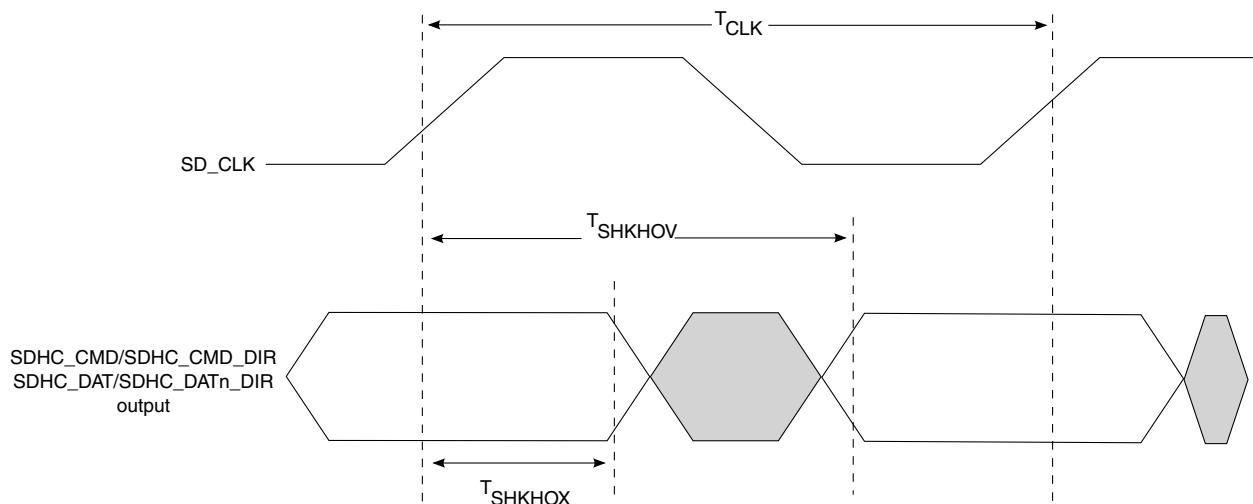
**Figure 19. eSDHC SDR50 mode output timing diagram**
