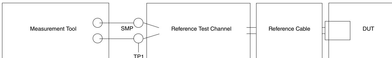
**Figure 94. Transmit normative setup**
