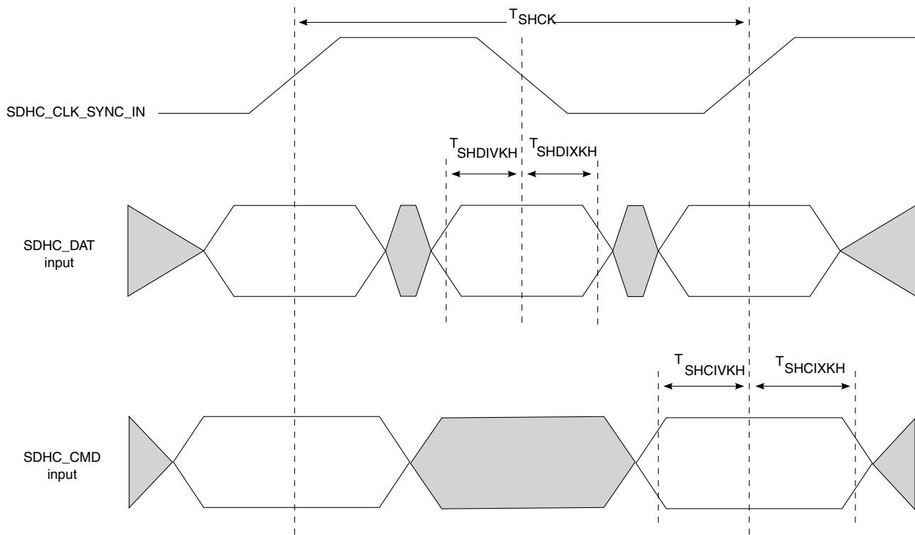
**Figure 20. eSDHC DDR50/DDR mode input AC timing diagram**
