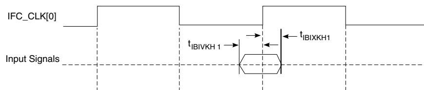
**Figure 48. IFC-GPCM, IFC-GASIC input AC timing specifications**
