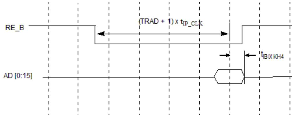
**Figure 67.  $t_{IBIXKH4}$  timings**
