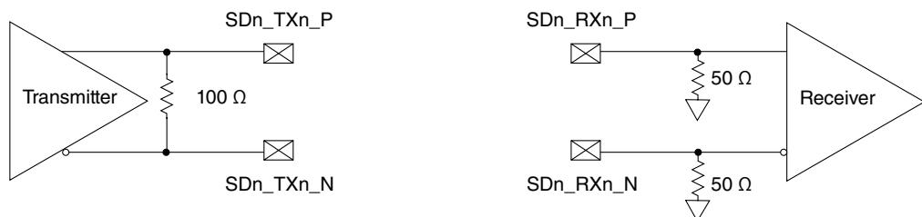
**Figure 36. SerDes transmitter and receiver reference circuits**
