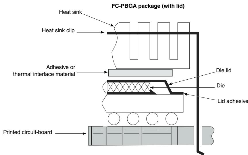
**Figure 95. Package exploded, cross-sectional view-FC-PBGA (with lid)**
