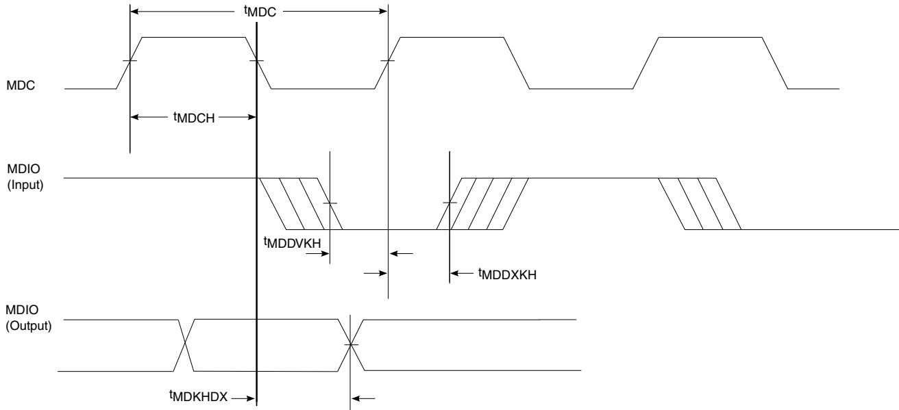
**Figure 24. Ethernet management interface 2 timing diagram**
