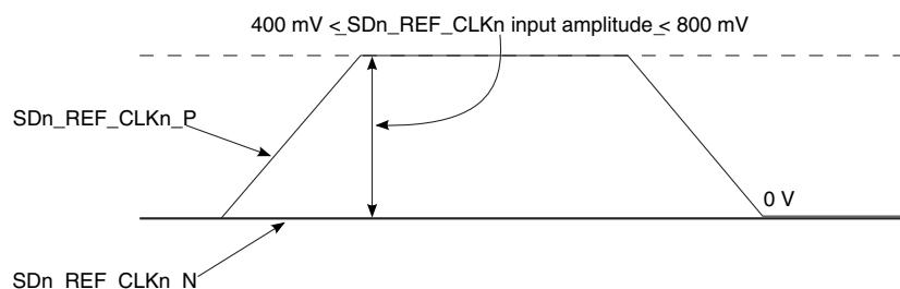
**Figure 33. Single-ended reference clock input DC requirements**
