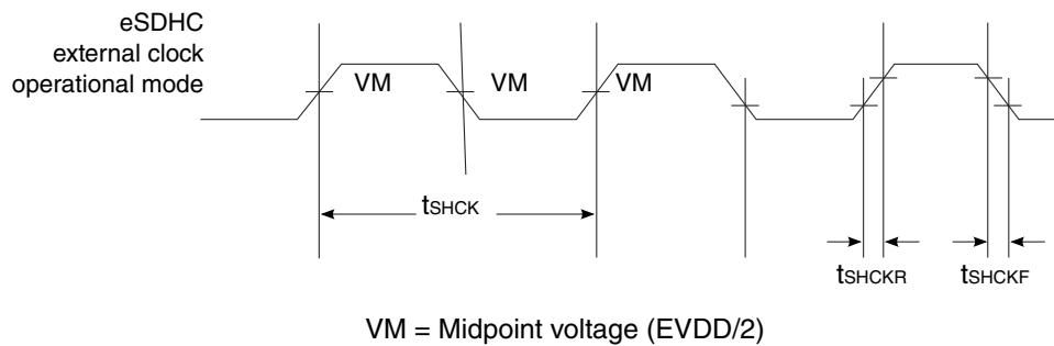
**Figure 17. eSDHC SDR50 mode clock input timing diagram**
