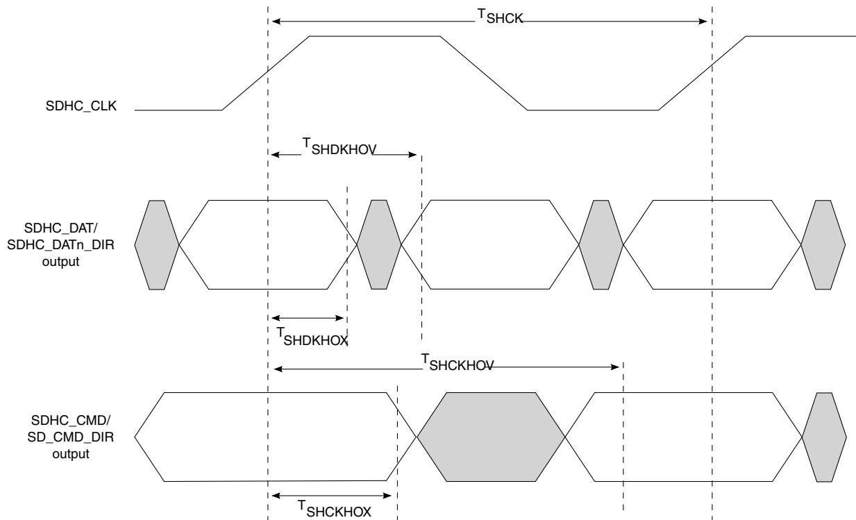
**Figure 21. eSDHC DDR50/DDR mode output AC timing diagram**
