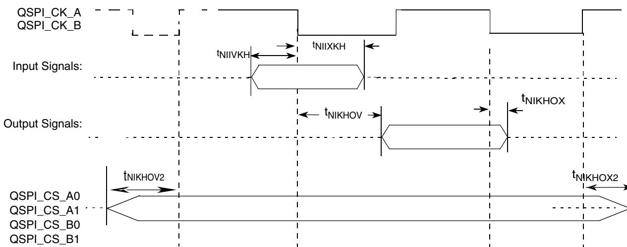
**Figure 82. QuadSPI AC timing — SDR mode**
