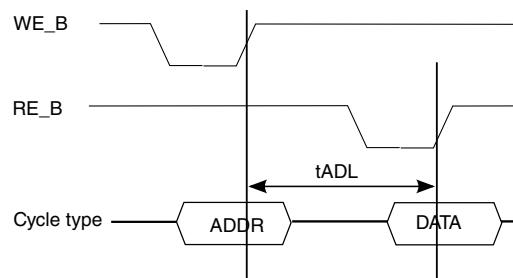
**Figure 54. t<sub>ADL</sub> timing**
