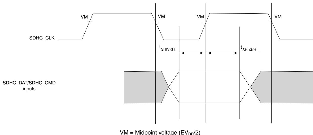
**Figure 15. eSDHC high-speed mode input AC timing diagram**
