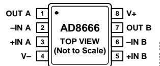
Figure 4. AD8666, 8-Lead MSOP (RM-8)
