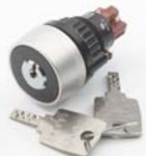
Keylock switch, 2 position, raised, gold over silver contacts, solder terminals, snap-action
