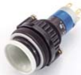
Illuminated pushbutton actuator for raised and flush mount, black plastic, plug-in terminal, snap-action, gold over silver contacts
