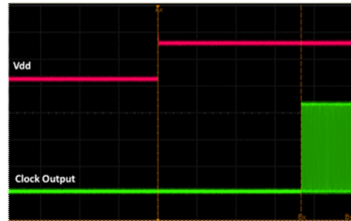
Figure 16. Startup Waveform vs. Vdd
