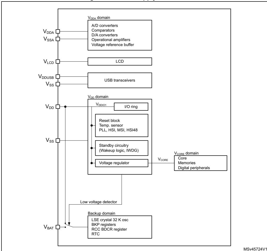
During power-up and power-down phases, the following power sequence requirements must be respected:
