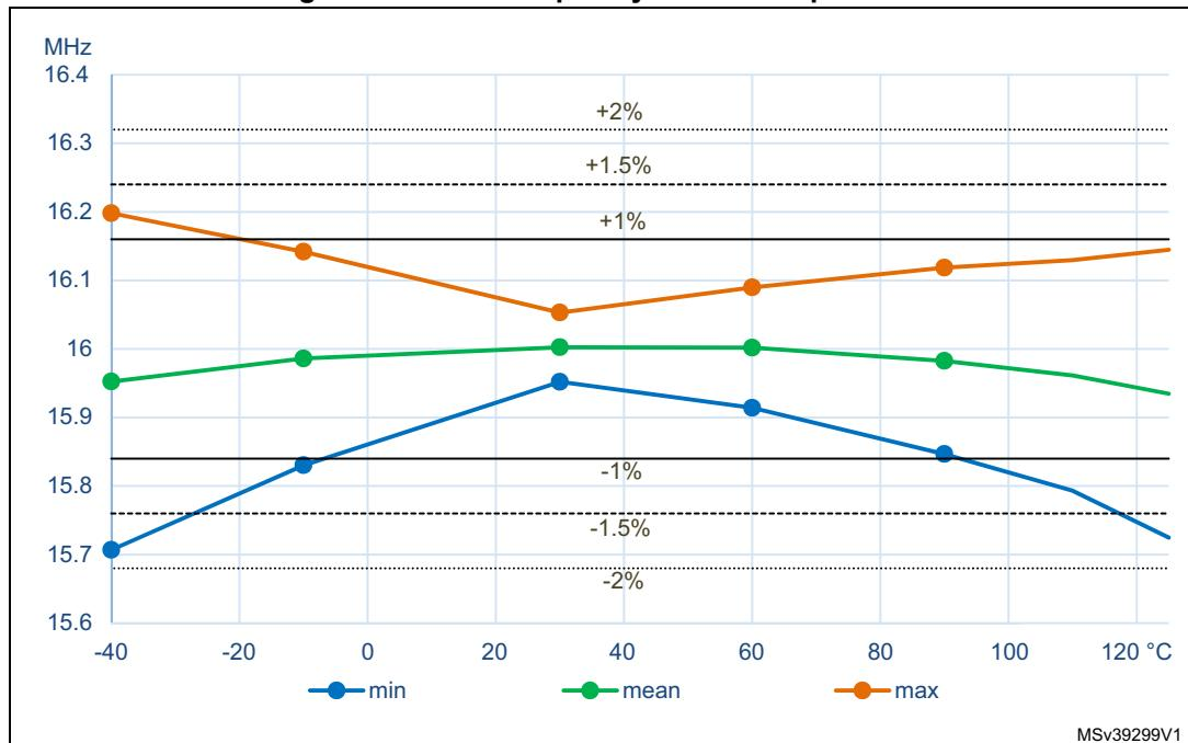
**Multi-speed internal (MSI) RC oscillator**Table 48. MSI oscillator characteristics<sup>(1)</sup>
