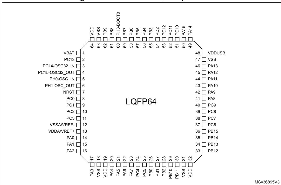
1. The above figure shows the package top view.
