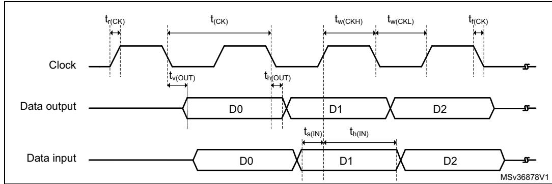
**Figure 37. Quad SPI timing diagram - DDR mode**
