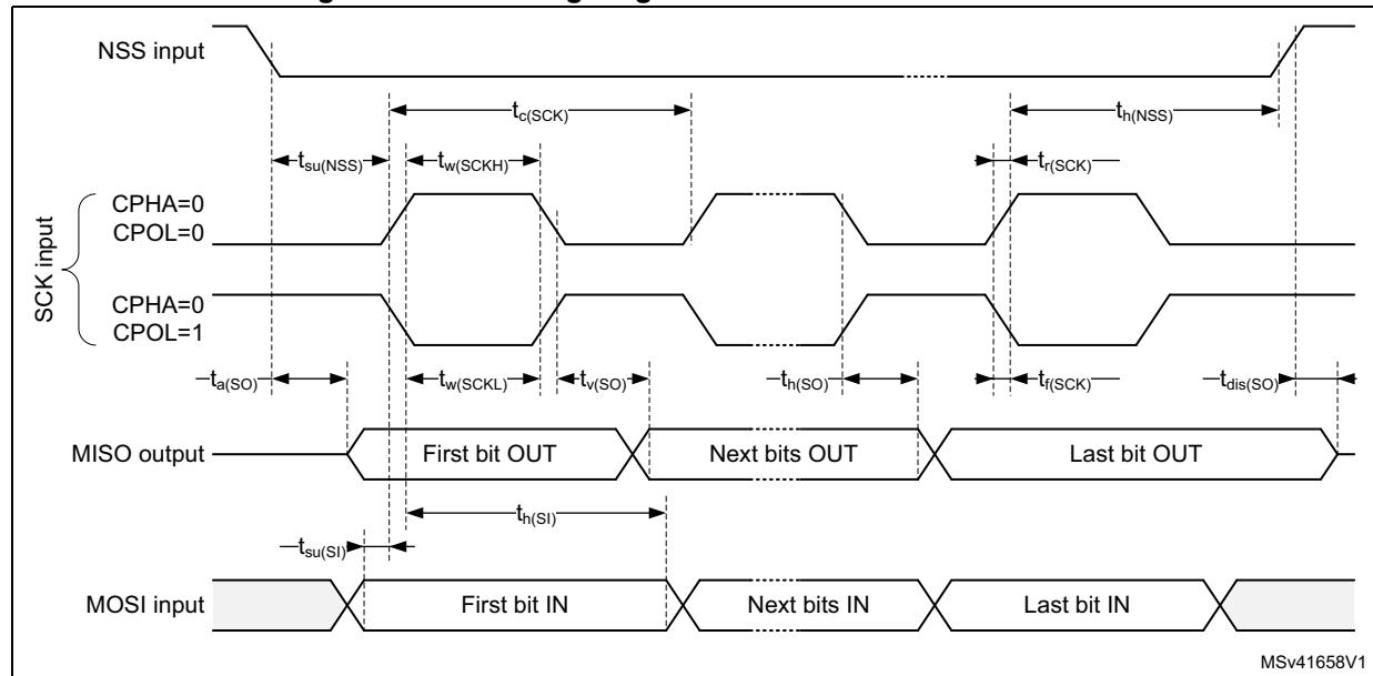
Figure 34. SPI timing diagram - slave mode and CPHA = 1
