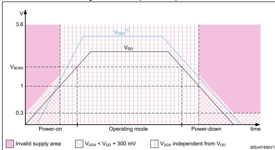
1.  $V_{DDX}$  refers to any power supply among  $V_{DDA}$ ,  $V_{DDUSB}$ ,  $V_{LCD}$ .
