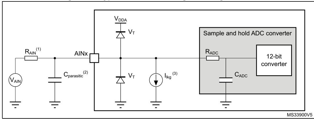
1. Refer to [Table 65: ADC characteristics](#) for the values of  $R_{AIN}$  and  $C_{ADC}$ .
