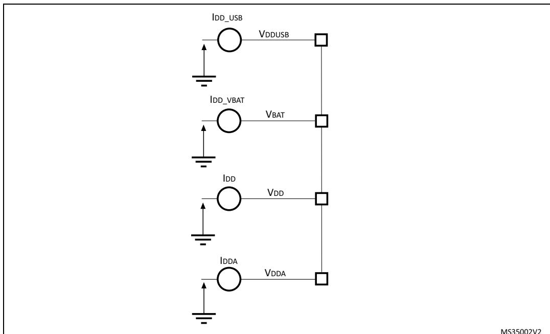
The  $I_{DD\_ALL}$  parameters given in [Table 25](#) to [Table 37](#) represent the total MCU consumption including the current supplying  $V_{DD}$ ,  $V_{DDA}$ ,  $V_{DDUSB}$  and  $V_{BAT}$ .
