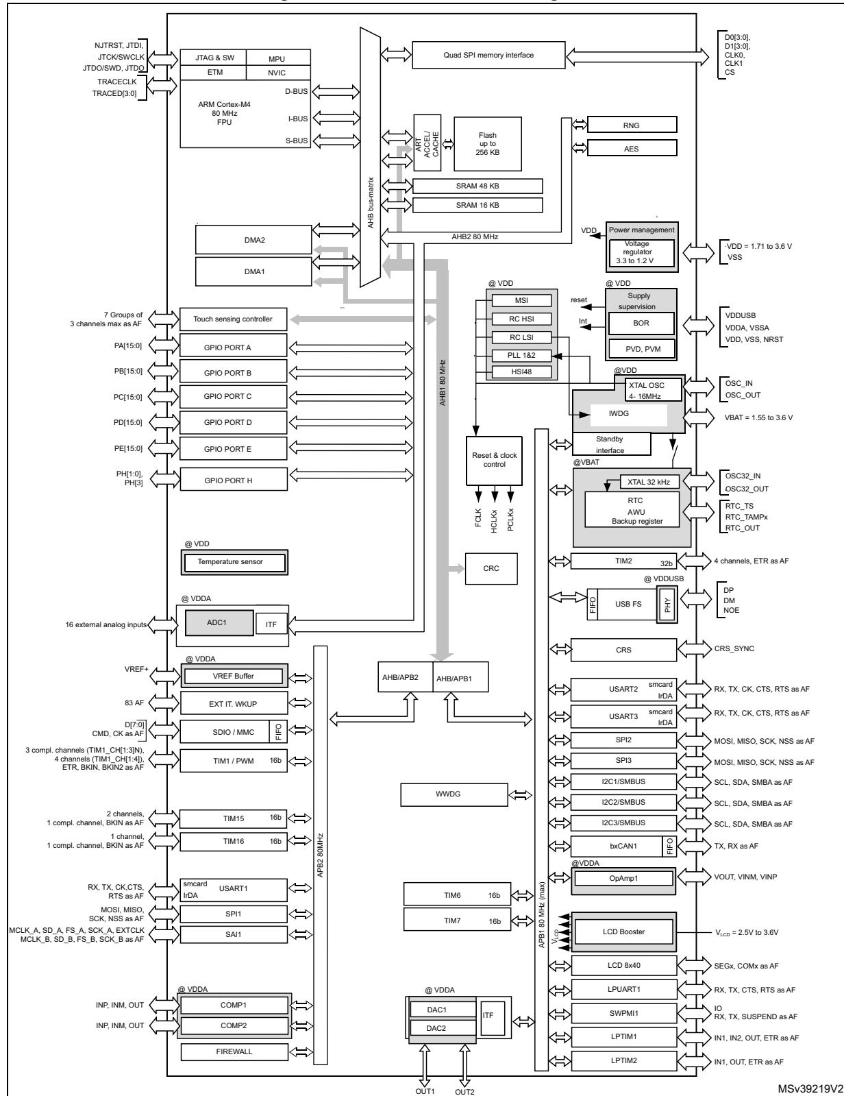
Note: AF: alternate function on I/O pins.
