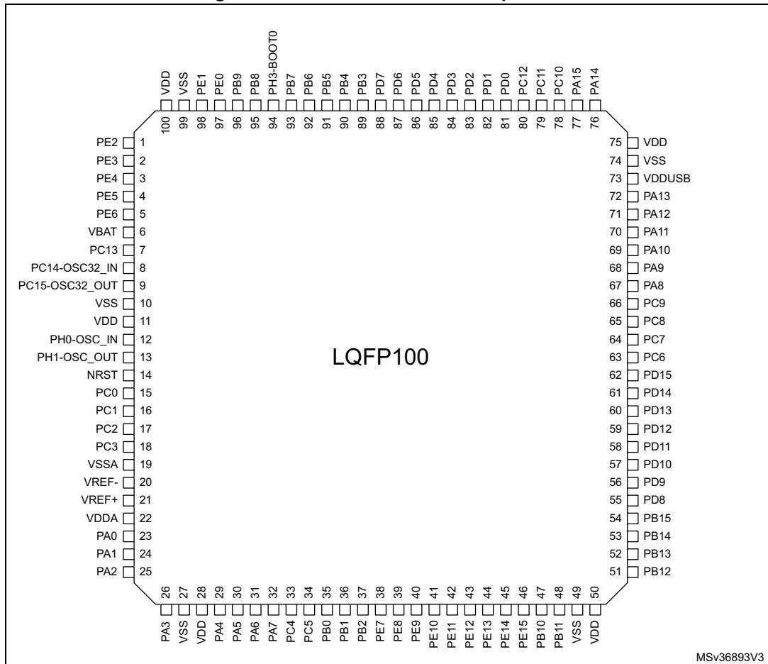
1. The above figure shows the package top view.
