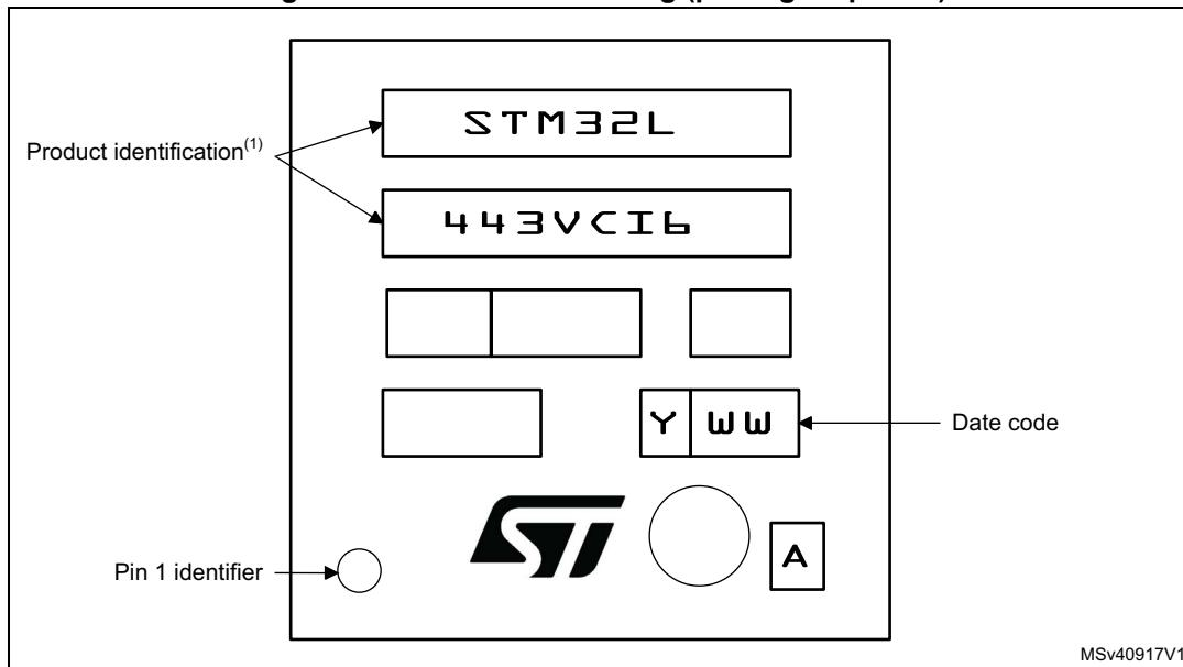
1. Parts marked as ES or E or accompanied by an Engineering Sample notification letter are not yet qualified and therefore not approved for use in production. ST is not responsible for any consequences resulting from such use. In no event will ST be liable for the customer using any of these engineering samples in production. ST's Quality department must be contacted prior to any decision to use these engineering samples to run a qualification activity.
