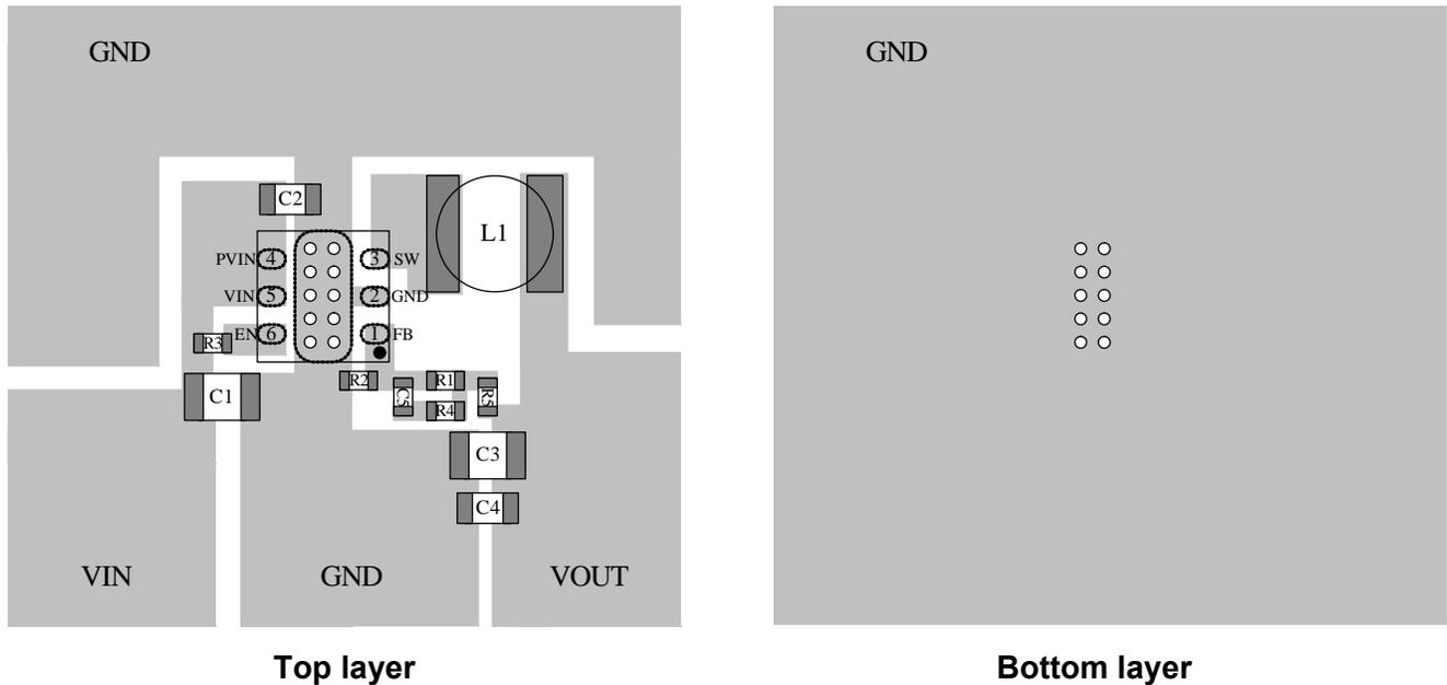
**Figure 3—PCB Layout**
