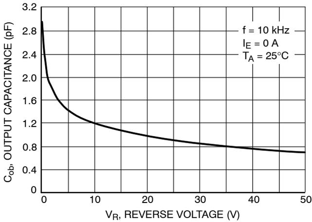
Figure 4. Output Capacitance
