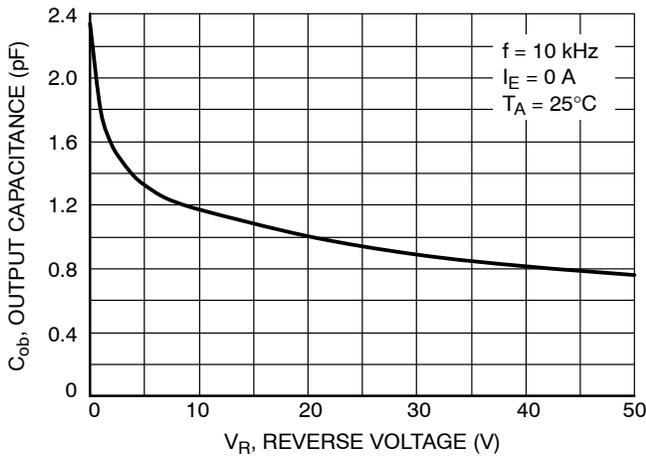
Figure 9. Output Capacitance
