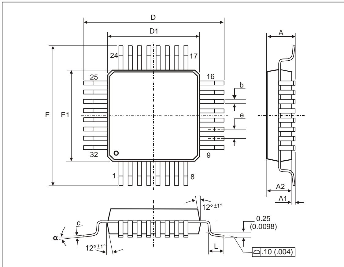
Fig. 6: LQFP32 (Low profile Quad Flat Package)
