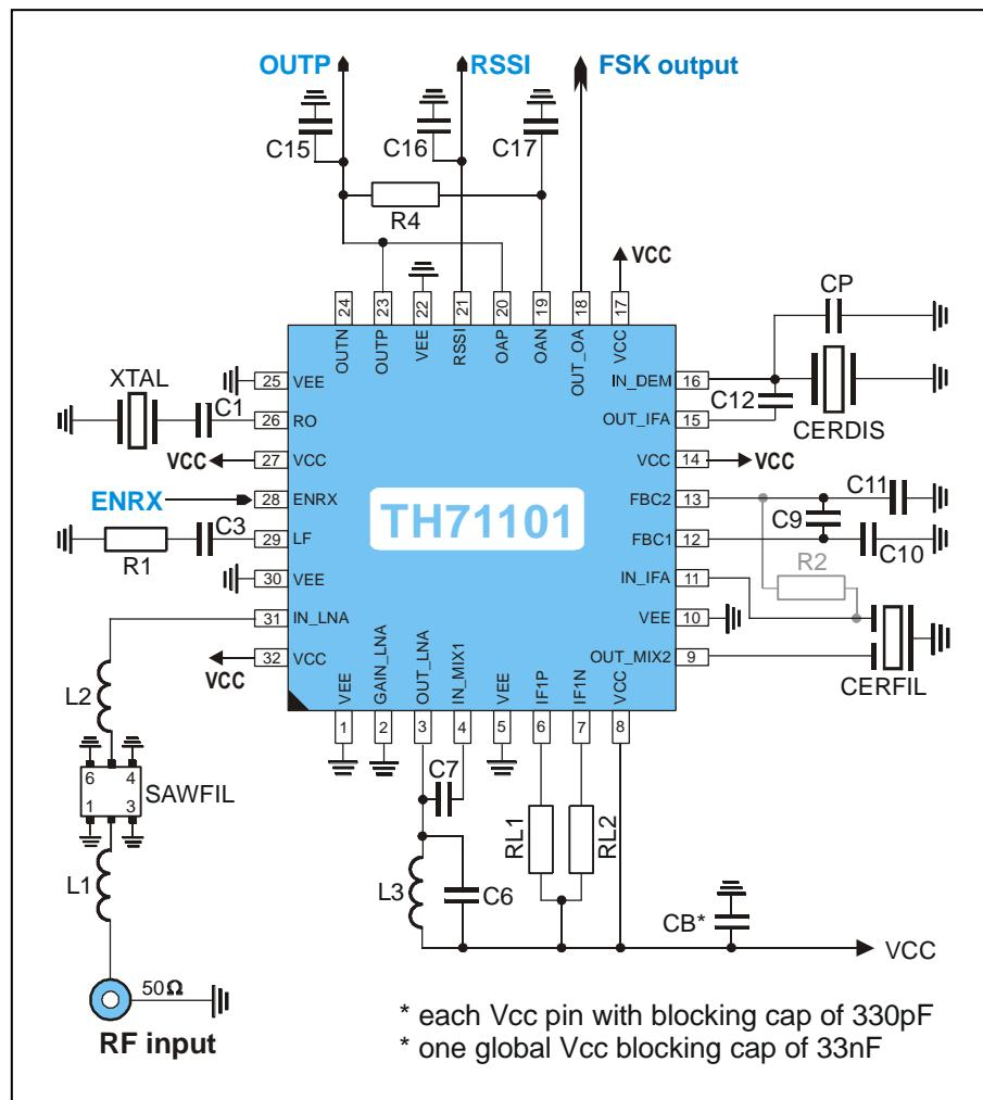
*Fig. 3: Test circuit for FSK reception (narrow band)*
