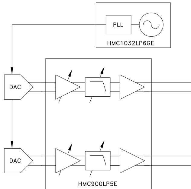
Figure 12. HMC1032LP6GE in a typical transmit chain
