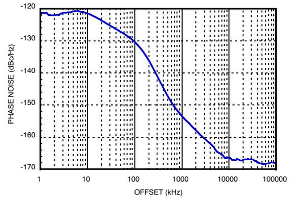
**Figure 3. Free Running Phase Noise [3]**
