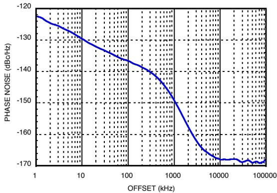
**Figure 2. Typical Closed Loop Fractional Phase Noise @ 312.5 MHz [2]**
