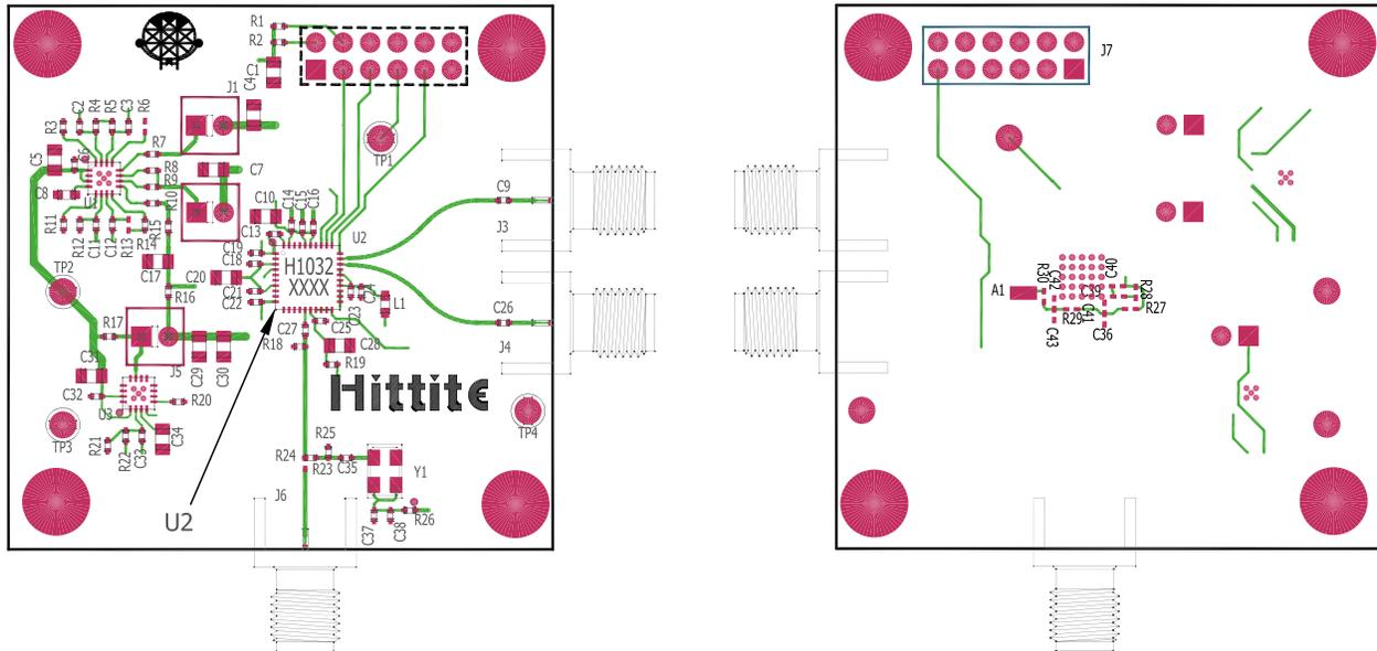
The circuit board used in the application should use RF circuit design techniques. Signal lines should have 50 Ohm impedance while the package ground leads and exposed paddle should be connected directly to the ground plane similar to that shown. A sufficient number of via holes should be used to connect the top and bottom ground planes. The evaluation circuit board shown is available from Hittite upon request.
