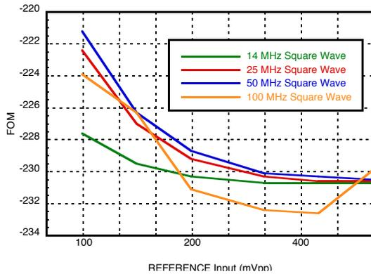
**Figure 8. Reference Input Sensitivity Sinusoid Wave [6]**
