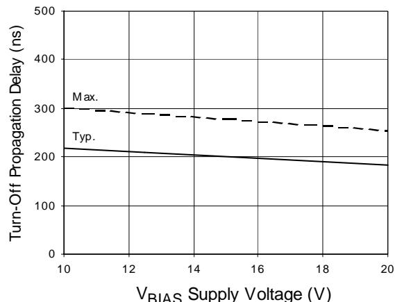
**Figure 5B. Turn-Off Propagation Delay vs. Supply Voltage**
