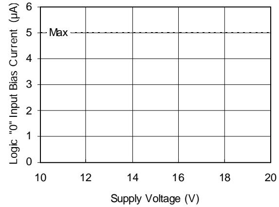
**Figure 16B.** Logic "0" Input Bias Current
