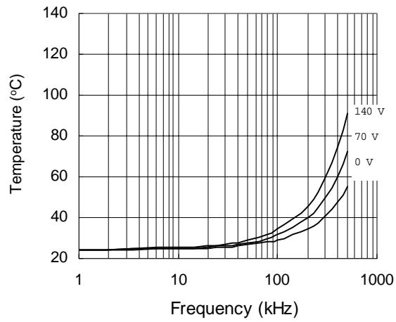
**Figure 30. IRS21064 vs. Frequency (IRFBC40),
