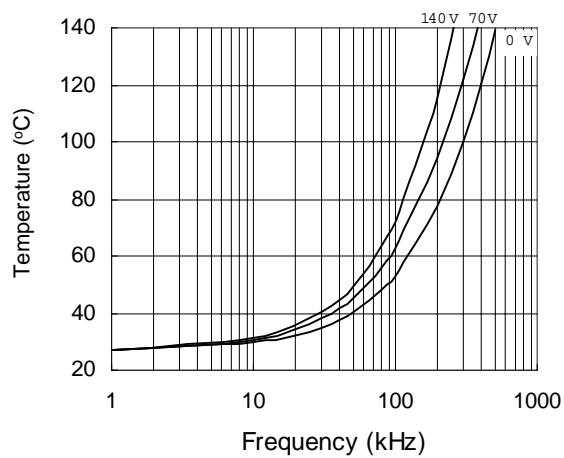
**Figure 39. IRS21064S vs. Frequency (IRFPE50),**
