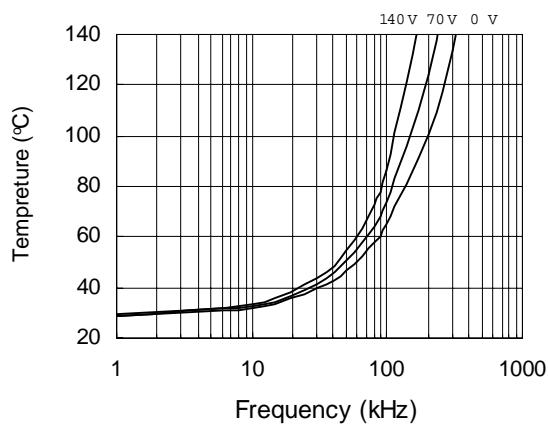
**Figure 35. IRS2106S vs. Frequency (IRFPE50),**
