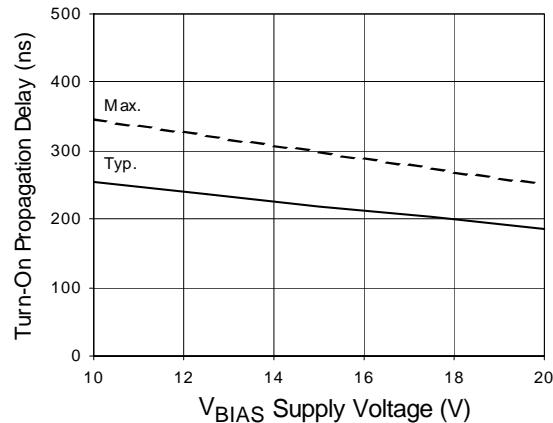
**Figure 4B. Turn-On Propagation Delay vs. Supply Voltage**
