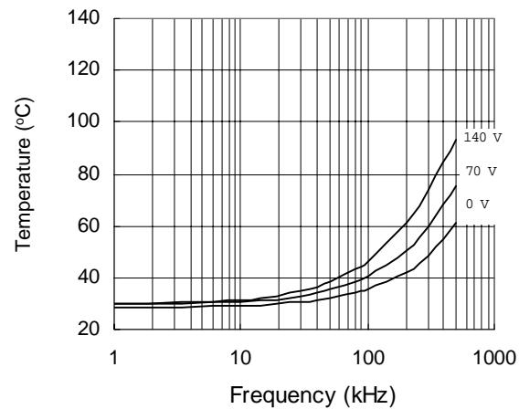
**Figure 26. IRS2106 vs. Frequency (IRFBC40),**
