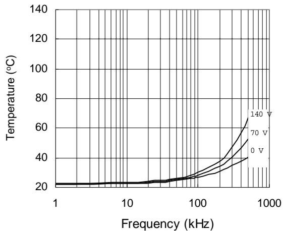
**Figure 29. IRS21064 vs. Frequency (IRFBC30),
