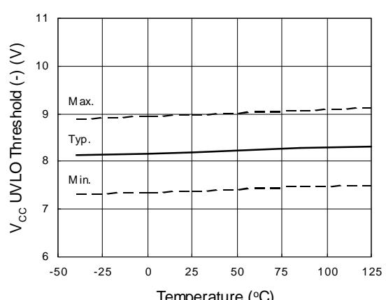
**Figure 18.**  $V_{\text{CC}}$  Undervoltage Threshold (-)
