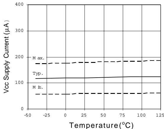
Figure 14A. Quiescent V<sub>CC</sub> Supply Current vs. Temperature
