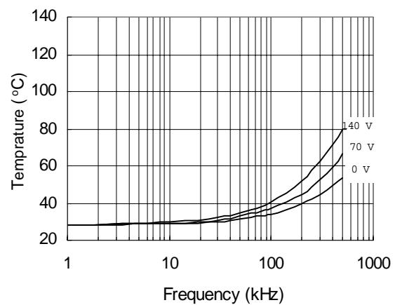
Figure 24. IRS2106 vs. Frequency (IRFB20), R<sub>gate</sub>=33 Ω, V<sub>CC</sub>=15 V
