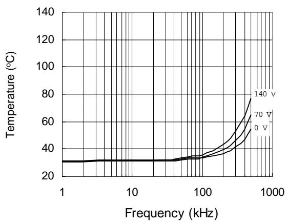
**Figure 32. IRS2106S vs. Frequency (IRFBC20),
