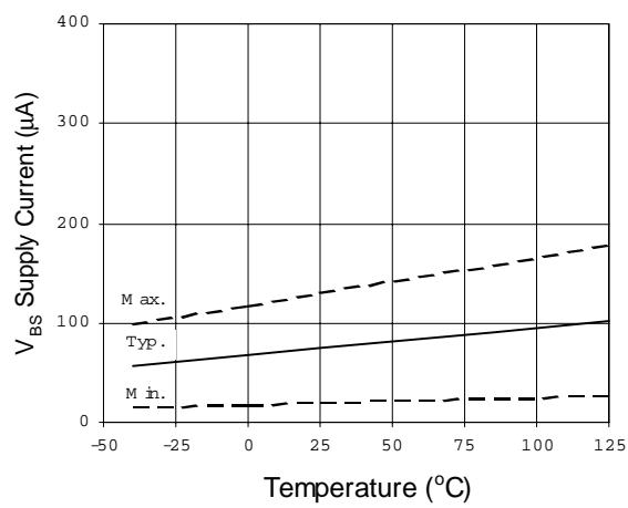
**Figure 13A. V<sub>BS</sub> Supply Current vs. Temperature**
