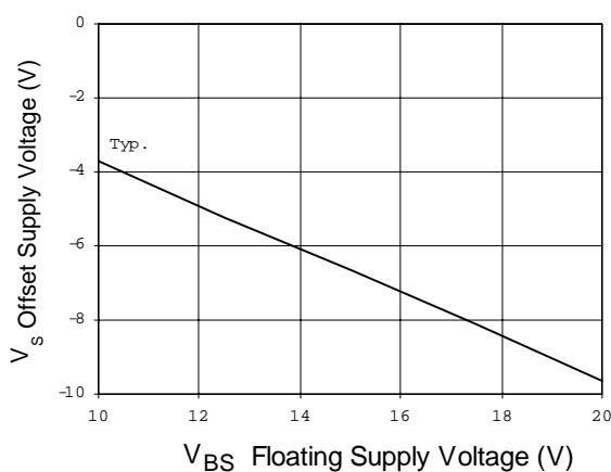
Figure 23. Maximum V<sub>S</sub> Negative Offset vs. Supply Voltage
