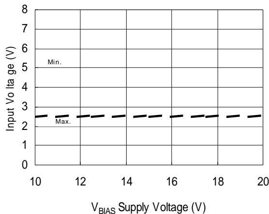
**Figure 8B. Logic "1" Input Voltage vs. Supply Voltage**
