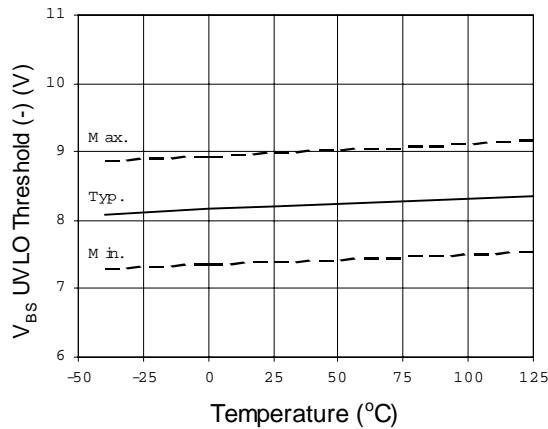
**Figure 20.  $V_{BS}$  Undervoltage Threshold (-) vs. Temperature**
