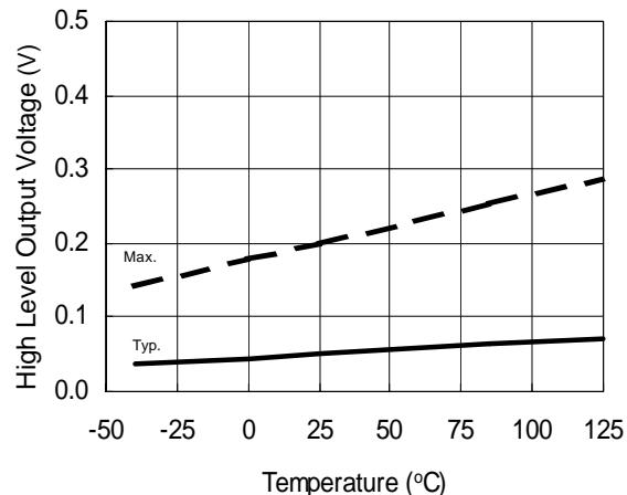
Figure 10A. High Level Output Voltage vs. Temperature
