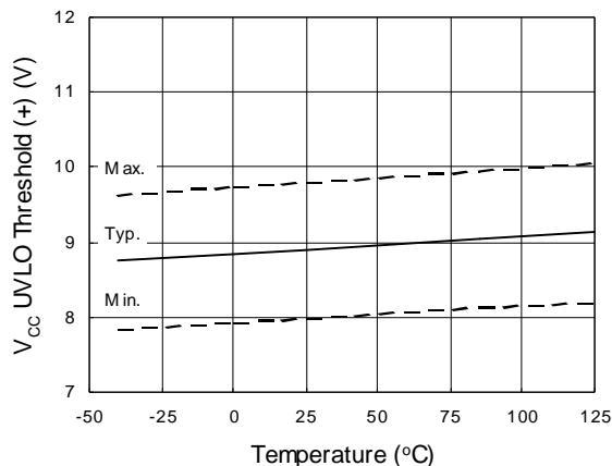
**Figure 17.**  $V_{\text{CC}}$  Undervoltage Threshold (+)
