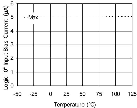
**Figure 16A.** Logic "0" Input Bias Current
