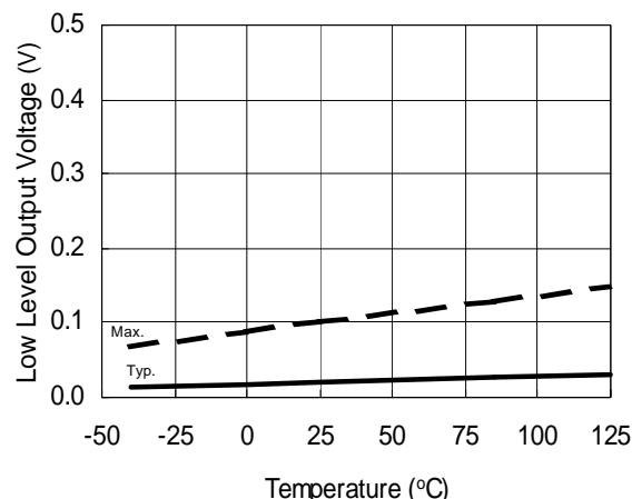
Figure 11A. Low Level Output Voltage vs. Temperature
