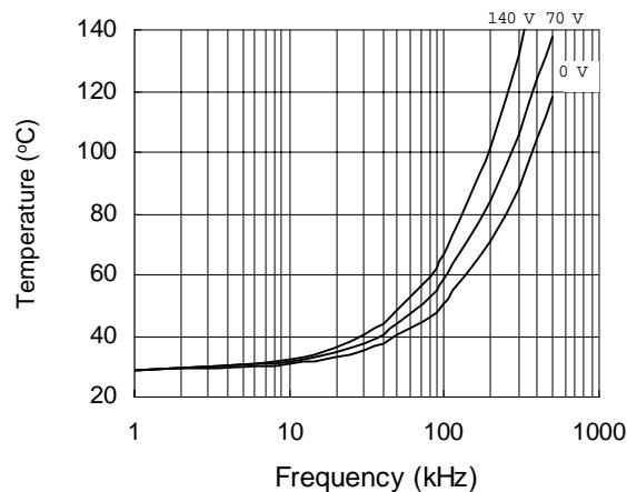
**Figure 27. IRS2106 vs. Frequency (IRFPE50),**
