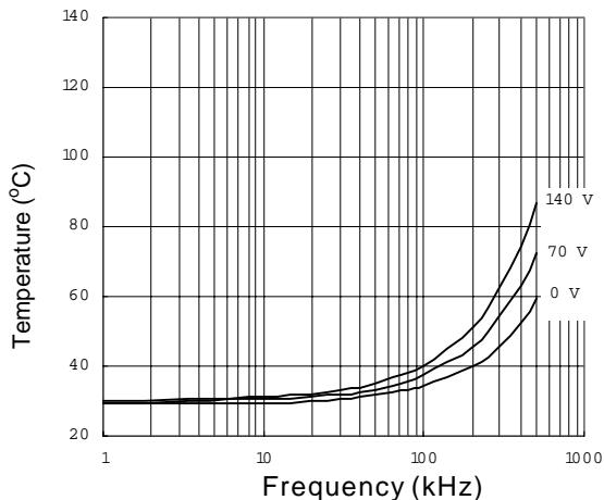
**Figure 25. IRS2106 vs. Frequency (IRFBC30),**
