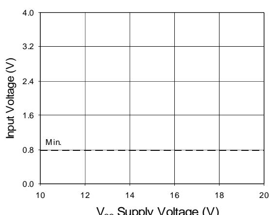
**Figure 9B. Logic "0" Input Voltage vs. Supply Voltage**
