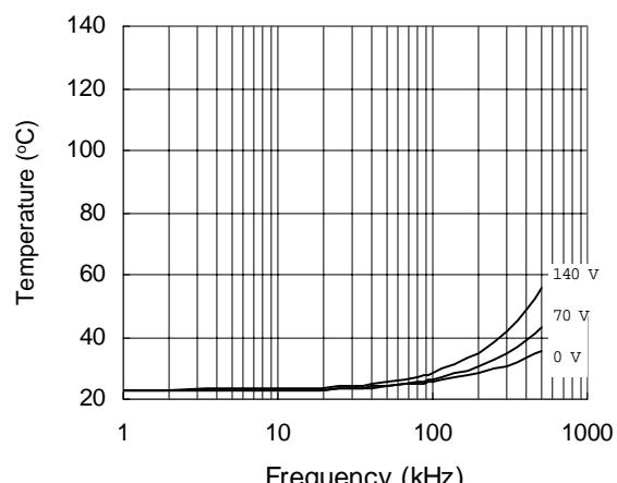
**Figure 28. IRS21064 vs. Frequency (IRFBC20),**
