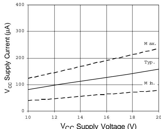
Figure 14B. Quiescent V<sub>CC</sub> Supply Current vs. V<sub>CC</sub> Supply Voltage
