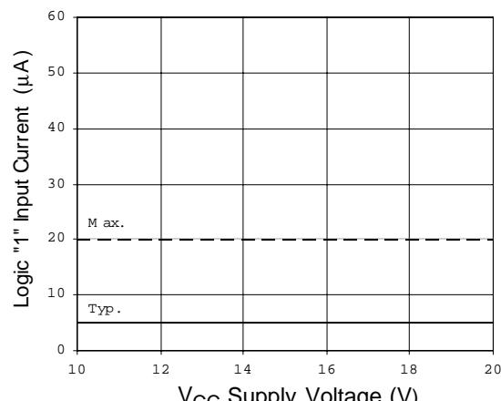
Figure 15B. Logic "1" Bias Current vs. Supply Voltage
