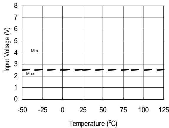
**Figure 8A. Logic "1" Input Voltage vs. Temperature**
