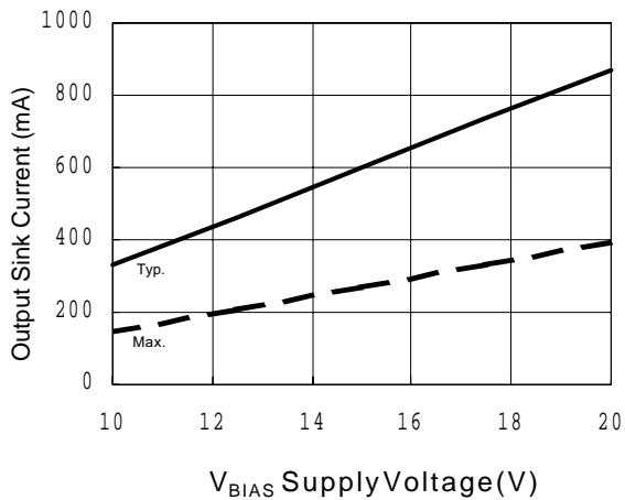
Figure 22B. Output Sink Current vs. Supply Voltage
