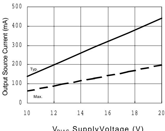
**Figure 21B. Output Source Current vs. Supply Voltage**
