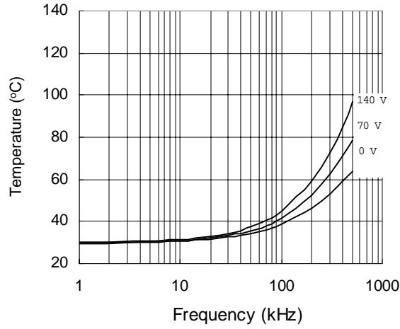
**Figure 38. IRS21064S vs. Frequency (IRFBC40),**
