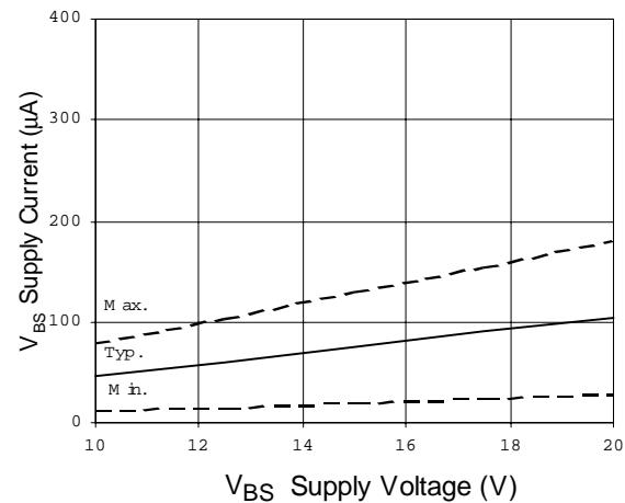
**Figure 13B. V<sub>BS</sub> Supply Current vs. Supply Voltage**
