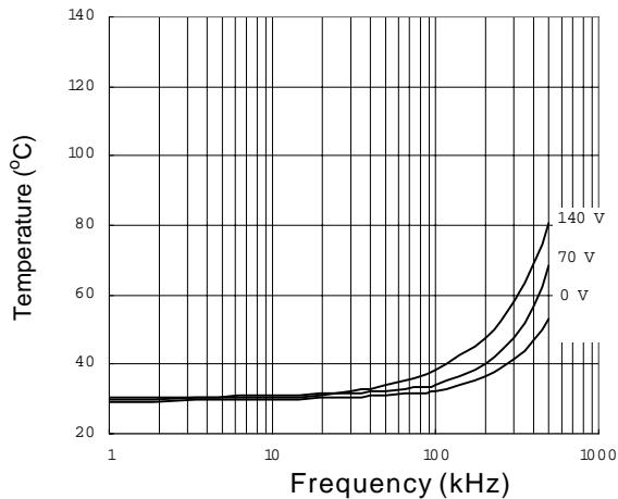
**Figure 37. IRS21064S vs. Frequency (IRFBC30),**
