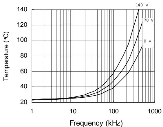
**Figure 31. IRS21064 vs. Frequency (IRFPE50),
