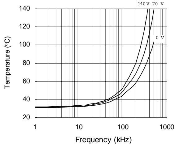
**Figure 34. IRS2106S vs. Frequency (IRFBC40),**
