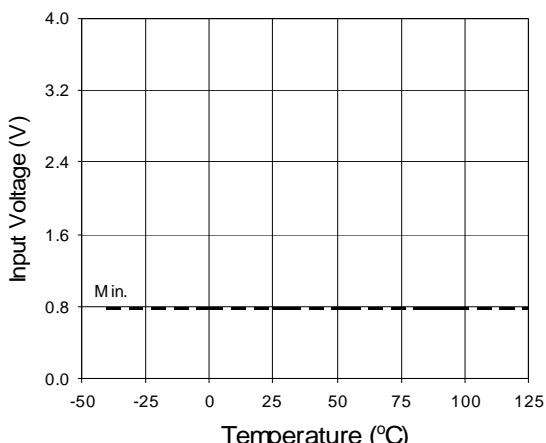
**Figure 9A. Logic "0" Input Voltage vs. Temperature**
