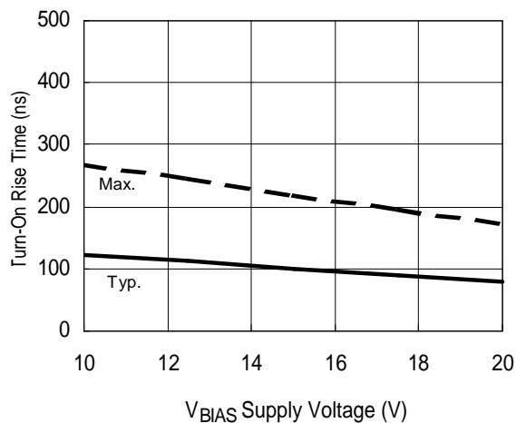
**Figure 6B. Turn-On Rise Time vs. Supply Voltage**
