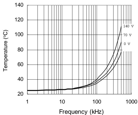
**Figure 33. IRS2106S vs. Frequency (IRFBC30),**
