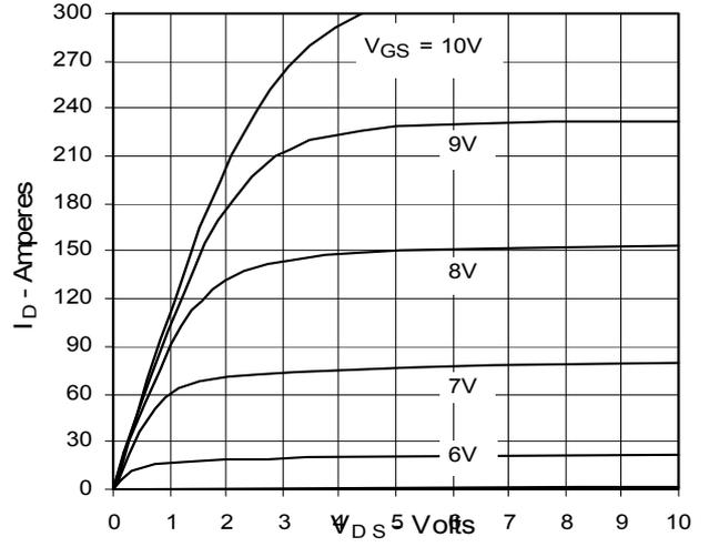
**Fig. 3. Output Characteristics**
