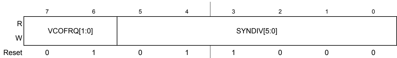
Figure 7-5. S12CPMU_UHV_V5 Synthesizer Register (CPMUSYNR)
