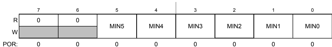
Figure 18-11. Minute Register (MINR)
