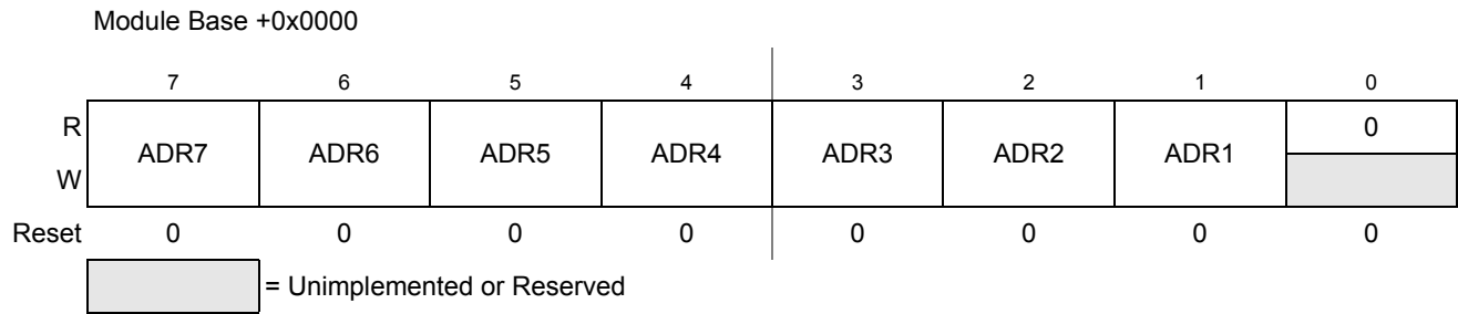
Figure 14-3. IIC Bus Address Register (IBAD)
