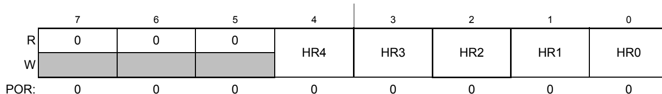
Figure 18-12. Hour Register (HRR)
