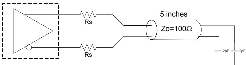
Note: The device can drive transmission line lengths greater than those allowed by the PCIe SIG.
