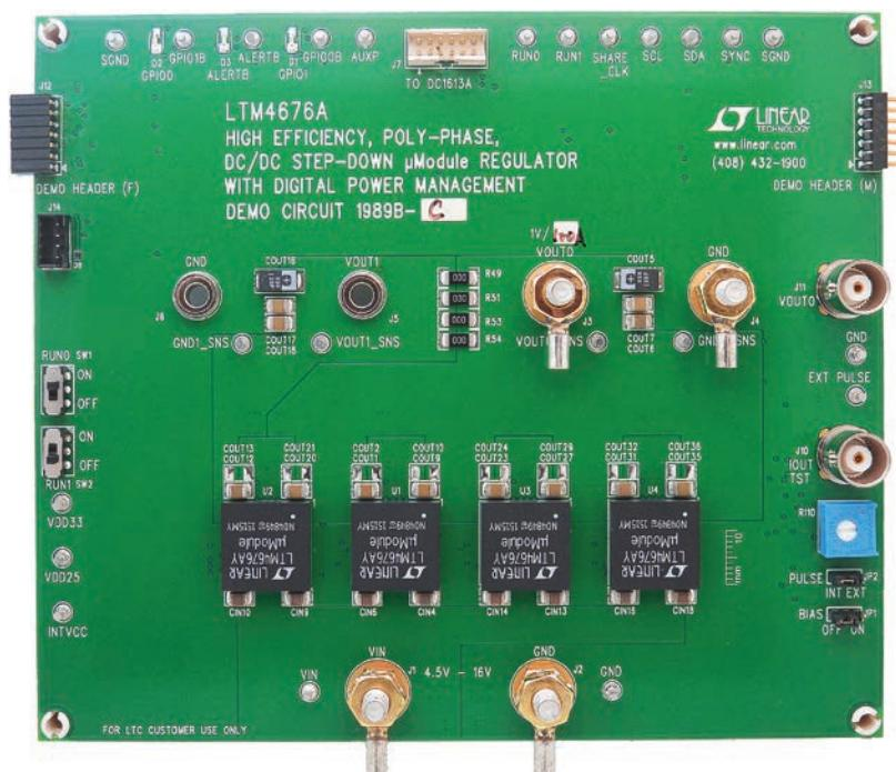
**Figure 1.** 4x LTM4676A: 100A DC1989B-C Demo Circuit
