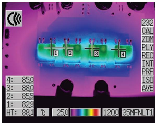
**Figure 8. Thermal Performance at  $V_{IN} = 12V$ ,  $V_{OUT0} = 1V$ ,  $I_{OUT0} = 100A$ ,  $T_A = 23.8^{\circ}C$ , Air Flow 300LFM**
