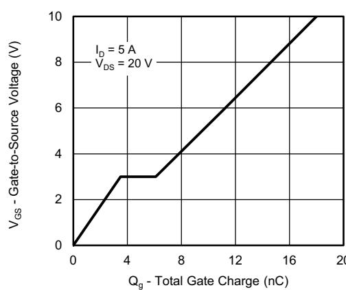
**N-CHANNEL TYPICAL CHARACTERISTICS ( $T_A = 25^\circ\text{C}$ , unless otherwise noted)**
