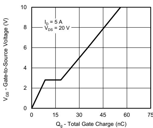
**P-CHANNEL TYPICAL CHARACTERISTICS** ( $T_A = 25^\circ\text{C}$ , unless otherwise noted)
