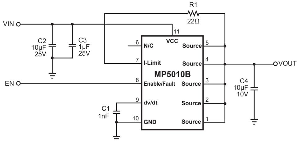
**Figure 5: Typical Application Schematic with Direct Current Sensing**
