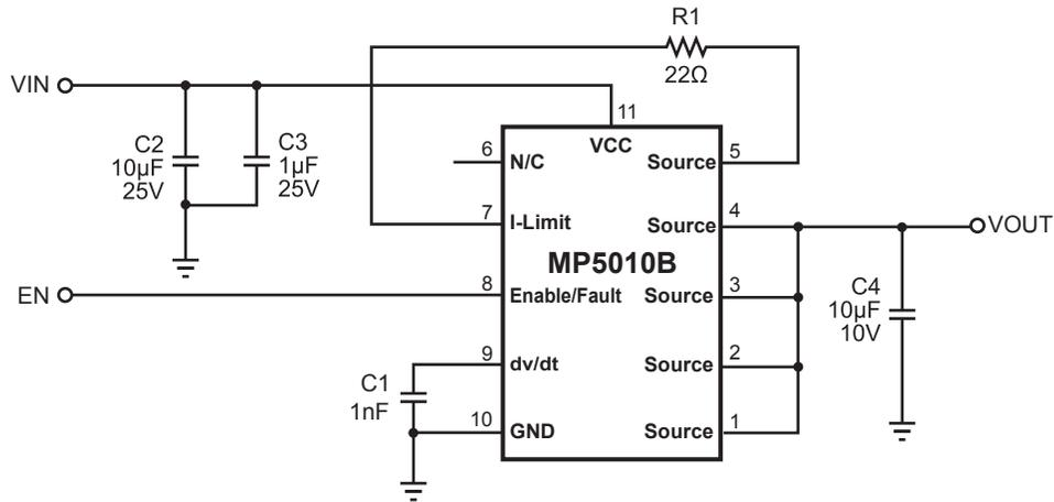
**Figure 4: Typical Application Schematic with Kelvin Current Sensing**
