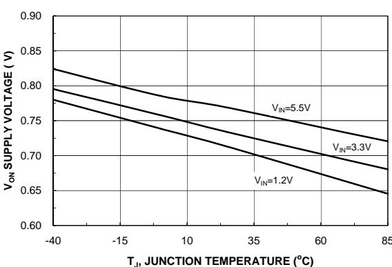
Figure 6. V<sub>ON</sub> High Voltage vs. Temperature
