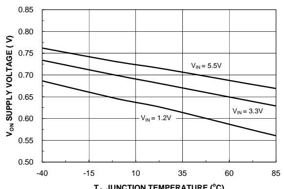
Figure 5. V<sub>ON</sub> Low Voltage vs. Temperature
