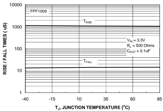
Figure 14. FPF1009  $t_{RISE}$  /  $t_{FALL}$  vs. Temperature
