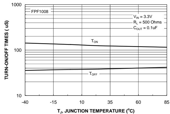
Figure 10. FPF1008  $t_{ON}$  /  $t_{OFF}$  vs. Temperature
