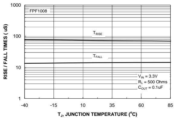
Figure 13. FPF1008  $t_{RISE}$  /  $t_{FALL}$  vs. Temperature
