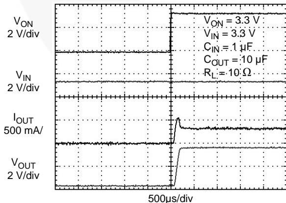
Figure 23. FPF1008 Turn-On Response ( $C_{OUT} = 10 \mu\text{F}$ )
