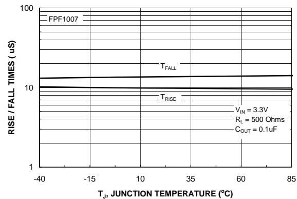
Figure 12. FPF1007  $t_{RISE}$  /  $t_{FALL}$  vs. Temperature
