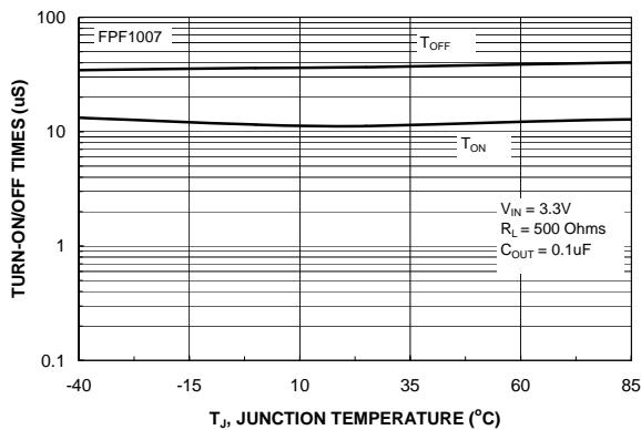
Figure 9. FPF1007  $t_{ON}$  /  $t_{OFF}$  vs. Temperature
