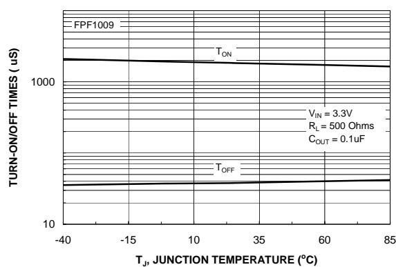
Figure 11. FPF1009  $t_{ON}$  /  $t_{OFF}$  vs. Temperature
