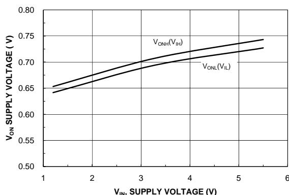
Figure 4. V<sub>ON</sub> Voltage vs. Input Voltage
