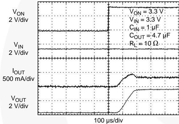
Figure 21. FPF1008 Turn-On Response ( $C_{OUT} = 4.7 \mu\text{F}$ )
