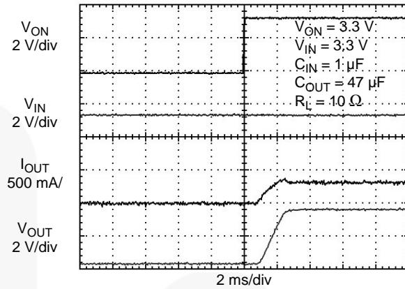
Figure 26. FPF1009 Turn-On Response ( $C_{OUT} = 47 \mu\text{F}$ )
