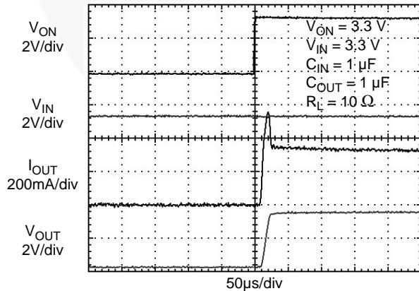
Figure 17. FPF1007 Turn-On Response ( $C_{OUT} = 1 \mu F$ )
