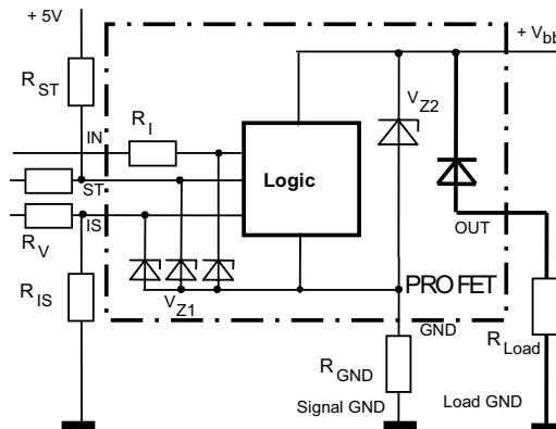
$V_{Z1} = 6.1 \text{ V typ.}$ ,  $V_{Z2} = 47 \text{ V typ.}$ ,  $R_{GND} = 150 \Omega$ ,
