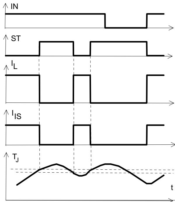
**Figure 5a:** Open load: detection (with  $R_{EXT}$ ),
