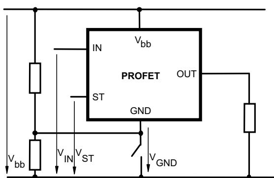
Any kind of load. If  $V_{GND} > V_{IN} - V_{IN(T+)}$  device stays off. Due to  $V_{GND} > 0$ , no  $V_{ST} = \text{low}$  signal available.
