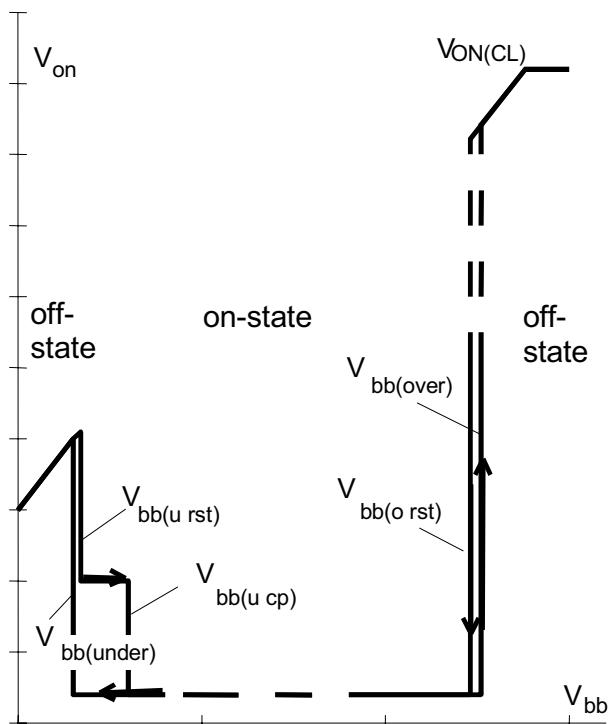
charge pump starts at  $V_{bb(\text{ucp})} = 4.7 \text{ V typ.}$
