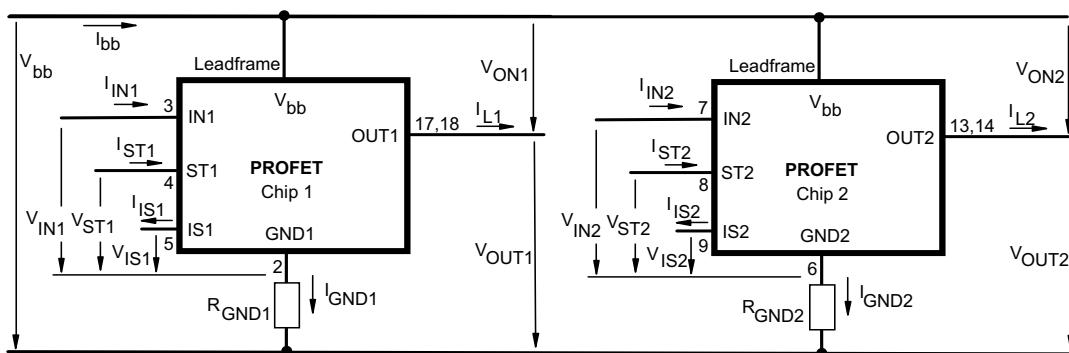
Leadframe ( $V_{bb}$ ) is connected to pin 1,10,11,12,15,16,19,20
