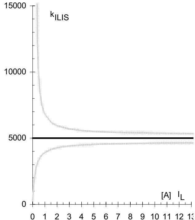
**Figure 8a:** Current sense versus load current<sup>26</sup>:
