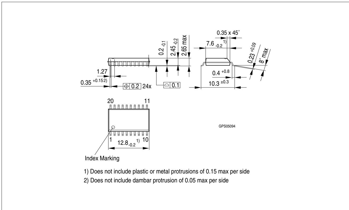
**Figure 1** PG-DSO-20 (Plastic Dual Small Outline Package) (RoHS-compliant)
