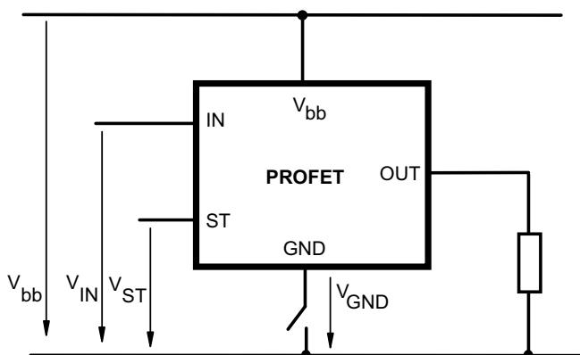
Any kind of load. In case of  $IN = \text{high}$  is  $V_{OUT} \approx V_{IN} - V_{IN(T+)}$ . Due to  $V_{GND} > 0$ , no  $V_{ST} = \text{low}$  signal available.
