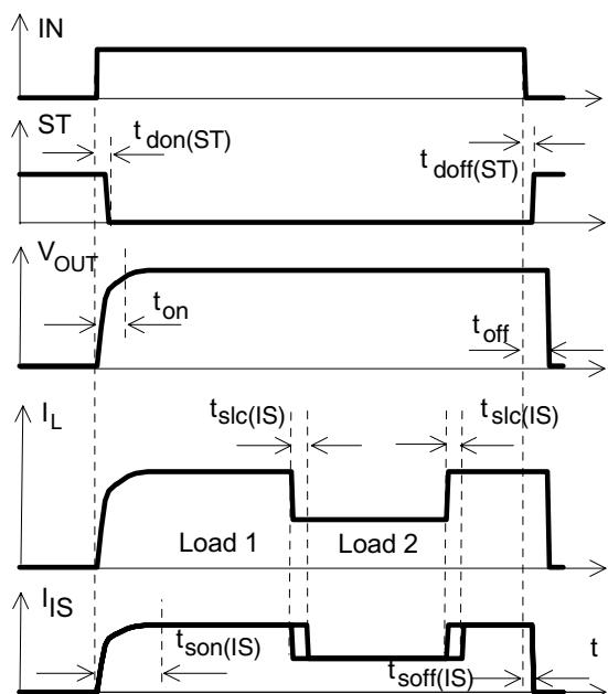
The sense signal is not valid during settling time after turn or change of load current.
