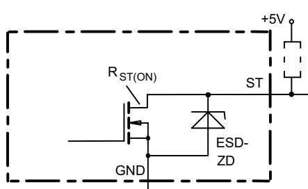
ESD-Zener diode: 6.1 V typ., max 5.0 mA;  $R_{ST(ON)} < 375 \Omega$  at 1.6 mA. The use of ESD zener diodes as voltage clamp at DC conditions is not recommended.
