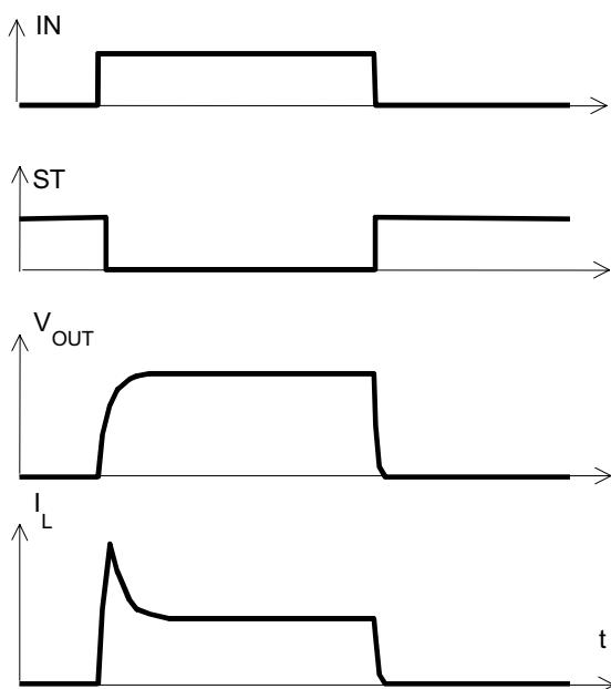
**Figure 2c:** Switching a lamp with current limit:
