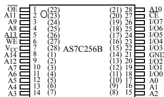
Note: This part is compatible with both pin numbering conventions used by various manufacturers.
