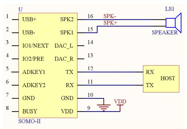
This example schematic shows a simple Serial connection to an external Host such as a 3.3V Microcontroller. It also shows the connections for an external speaker.
