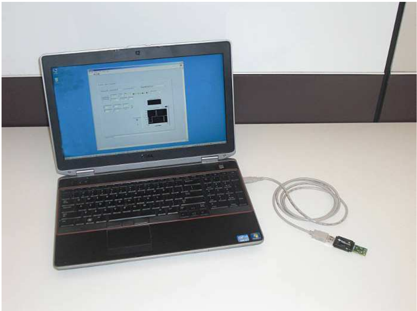
Figure 2. OPT3001EVM Hardware Setup
