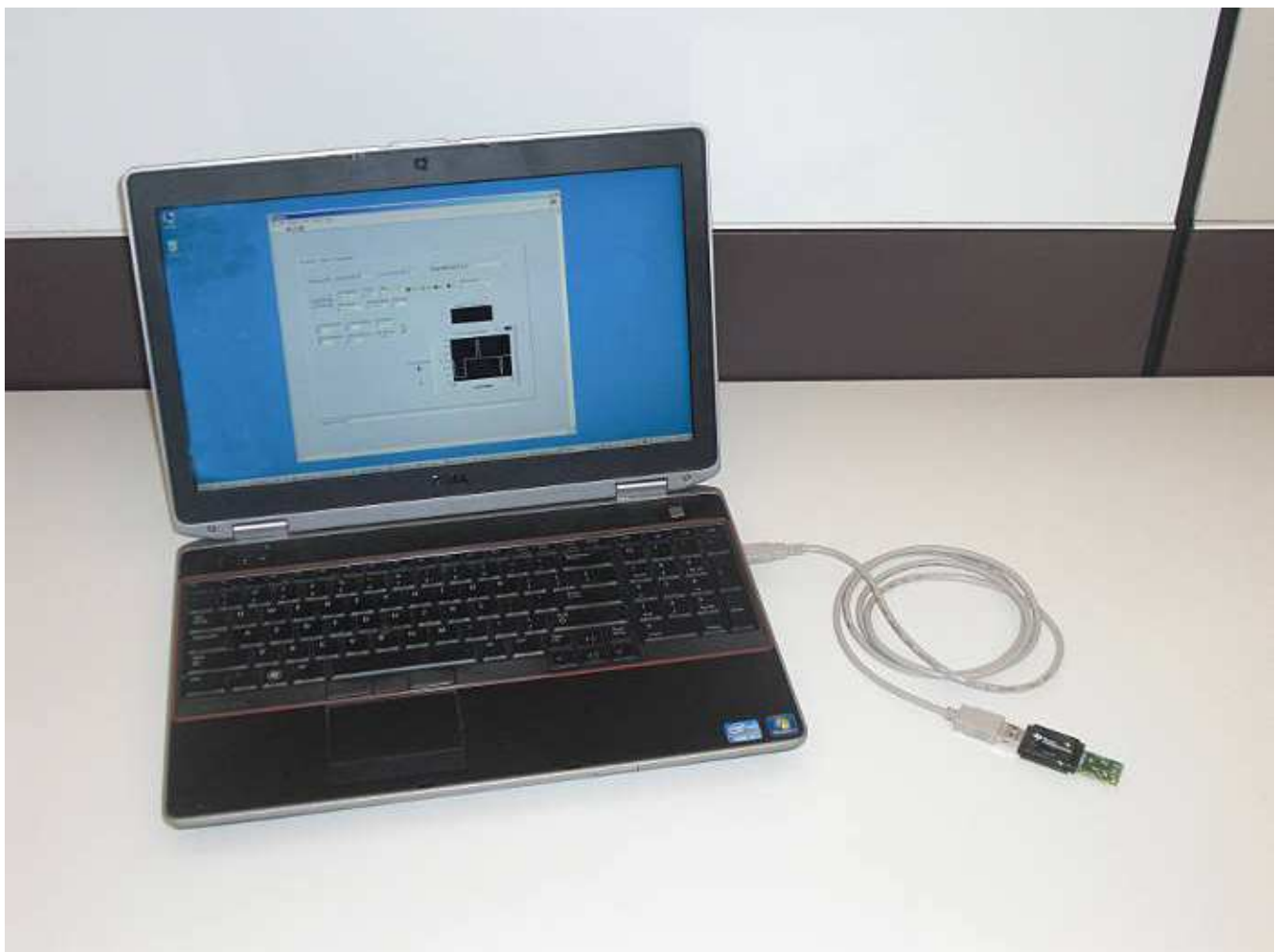
Figure 2. OPT3001EVM Hardware Setup
