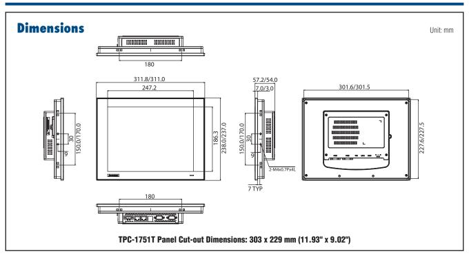
TPC-1751T-E3AE 17" SXGA Panel PC, Intel® Atom™ E3827 1.75 GHz Processor, 4GB (True-flat touch screen)
