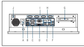
A. AC Power Input B.USB ports C. COM Ports
