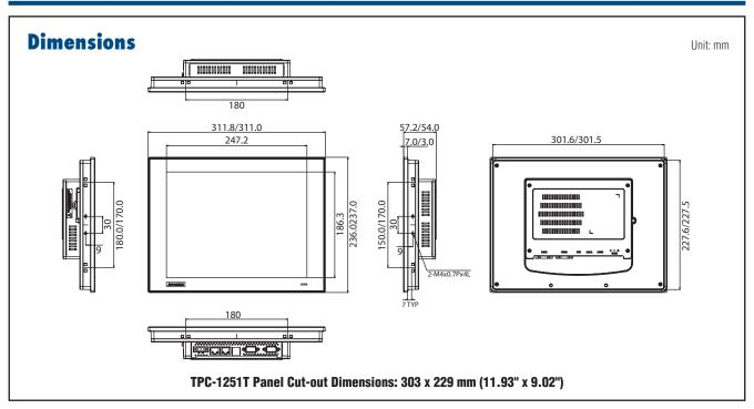
TPC-1251T-E3AE 12" XGA Panel PC. Intel® Atom™ E3827 1.75 GHz Processor, 4GB (True-flat touch screen)
