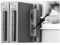
Node ID Setting 8-pin dip switch configuration
