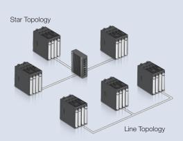
All APAX I/O modules are inserted on the backplane. Through the expansion port and Ethernet cable, different backplanes can be connected. This decentralized architecture retains high-speed data transfers, so the distributed I/O modules provide real-time performance. Almost any topology, such as line, tree or star, can be easily established. The hot swap capability is also available for remote expansion I/O modules.
