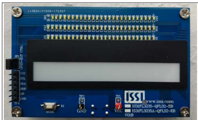
Figure 1: Photo of IS31FL3235/IS31FL3235A Evaluation Board
