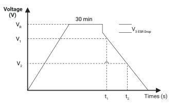
I - Discharge Current [mA], 4 \* C \* VR VR - Rated Voltage
