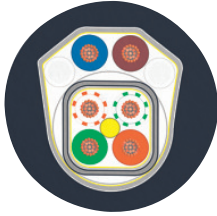
Cable cross section
