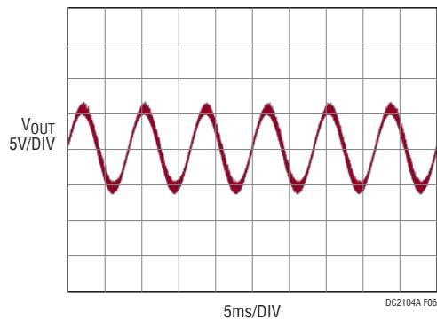
**Figure 6. Output Ripple (AC-Coupled), V<sub>IN</sub> = 115VAC**
