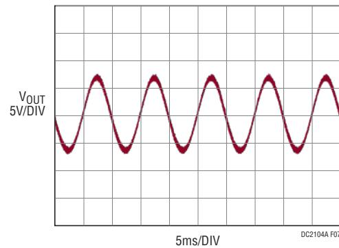
**Figure 7. Output Ripple (AC-Coupled), V<sub>IN</sub> = 230VAC**
