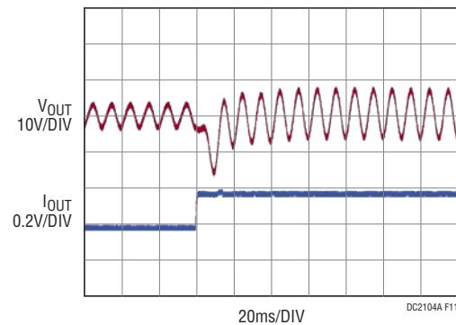
Figure 11.  $V_{IN} = 230\text{VAC}$ , Half Load to Full Load Transient
