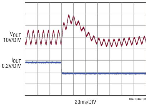
Figure 8.  $V_{IN} = 115\text{VAC}$ , Full Load to Half Load Transient
