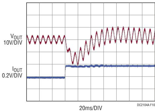
Figure 10.  $V_{IN} = 115\text{VAC}$ , Half Load to Full Load Transient
