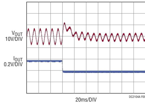
Figure 9.  $V_{IN} = 230\text{VAC}$ , Full Load to Half Load Transient
