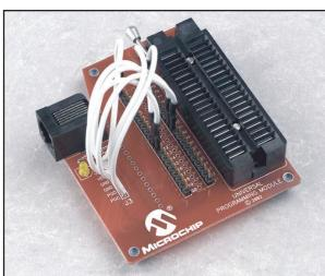
The Universal Programming Module can be used in conjunction with the MPLAB ICD 2 to provide an easy means for programming 300 to 600-mil PDIP Flash devices. It features a 40-pin ZIP socket, an MPLAB ICD 2 connector, programming indicator and configuration jumpers.
