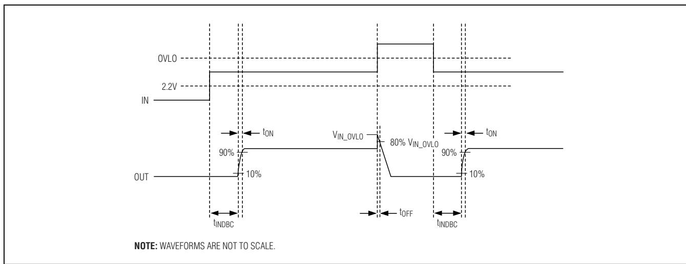
Figure 1. Timing Characteristics
