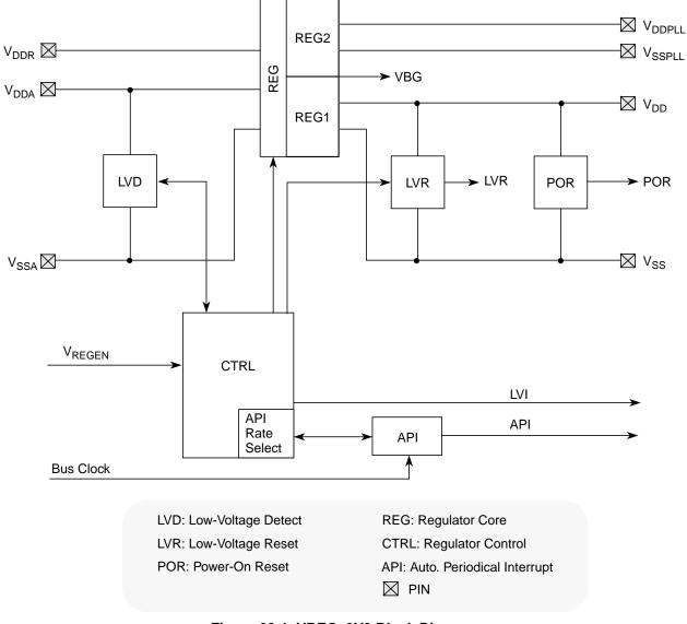
Figure 20-1. VREG\_3V3 Block Diagram
