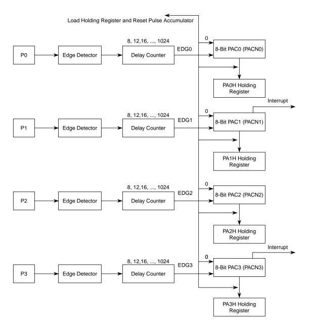
Figure 19-71. 8-Bit Pulse Accumulators Block Diagram
