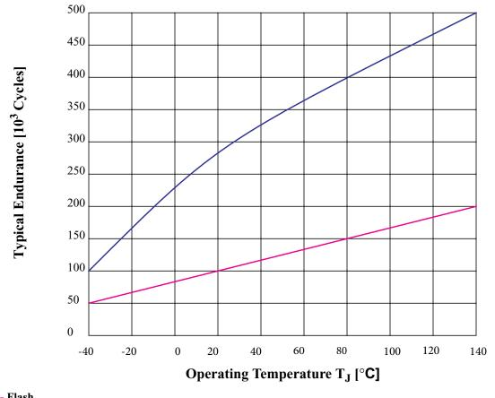
Figure A-2. Typical Endurance vs Temperature
