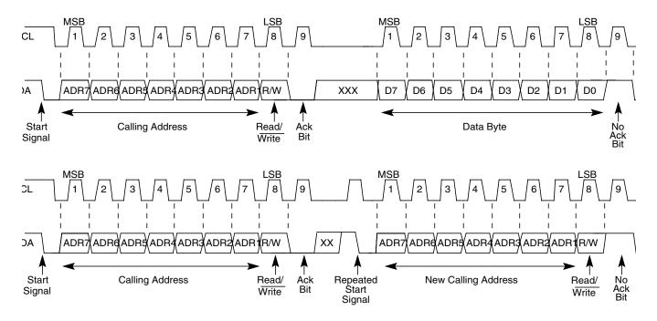
Figure 13-10. IIC-Bus Transmission Signals
