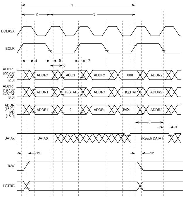
Figure A-14. Example 2b: Emulation Expanded Mode — Read with 1 Stretch Cycle
