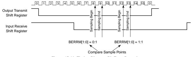
Figure 15-19. Timing Diagram Bit Error Detection
