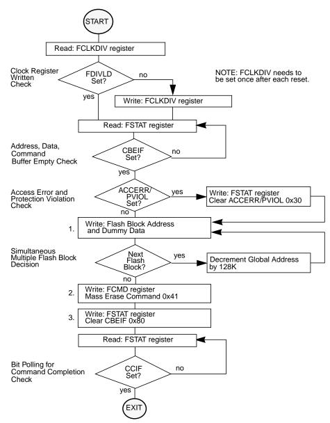
Figure 3-30. Example Mass Erase Command Flow
