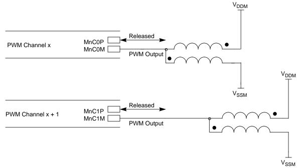
Figure 11-11. Typical Quad Half H-Bridge Mode Configuration
