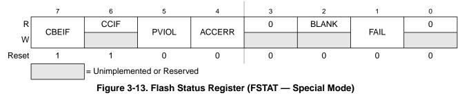
CBEIF, PVIOL, and ACCERR are readable and writable, CCIF and BLANK are readable and not writable, remaining bits read 0 and are not writable in normal mode. FAIL is readable and writable in special mode. FAIL must be clear in special mode when starting a command write sequence.
