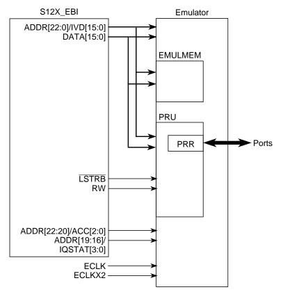
Figure 23-5. Application in Emulation Single-Chip Mode
