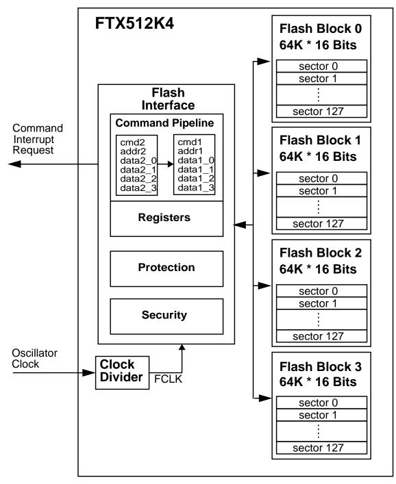
Figure 3-1. FTX512K4 Block Diagram
