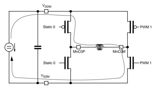
Figure 11-12. PWM Active Phase, RECIRC = 0, S = 0
