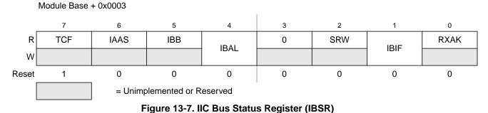
This status register is read-only with exception of bit 1 (IBIF) and bit 4 (IBAL), which are software clearable.
