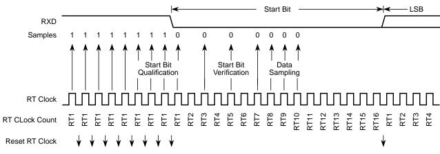
Figure 15-21. Receiver Data Sampling
