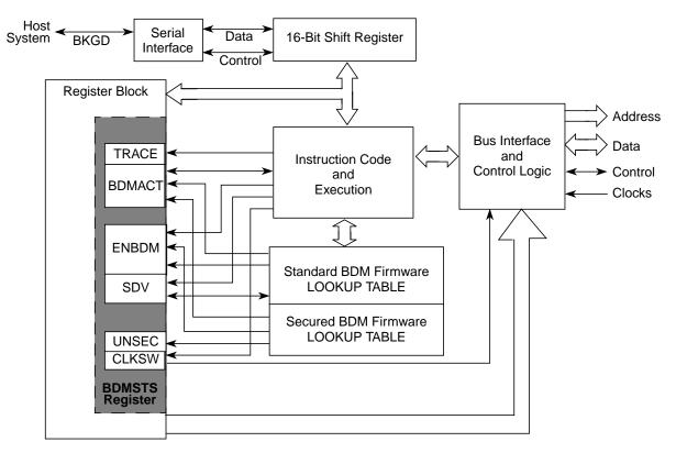
Figure 21-1. BDM Block Diagram
