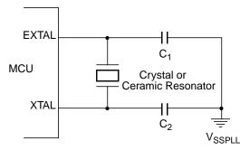
Figure 1-7. Loop Controlled Pierce Oscillator Connections (PE7 = 0)
