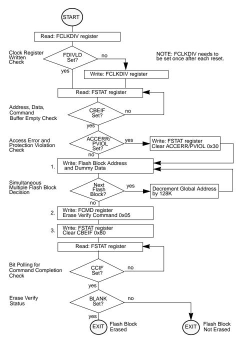
Figure 3-25. Example Erase Verify Command Flow
