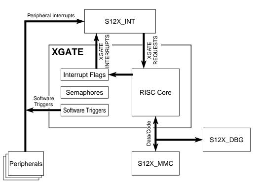
Figure 5-1. XGATE Block Diagram
