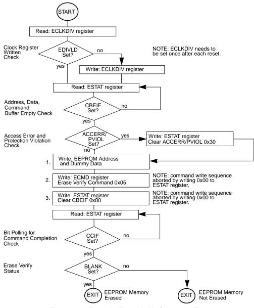
Figure 4-18. Example Erase Verify Command Flow
