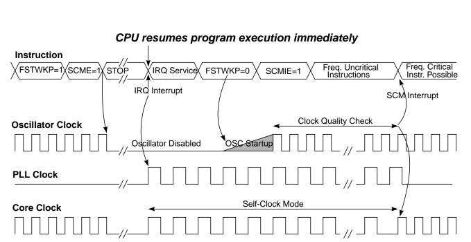
Figure 7-24. Fast Wake-up from Full Stop Mode: Example 2
