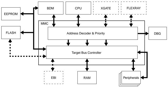
Figure 25-1. MMC Block Diagram
