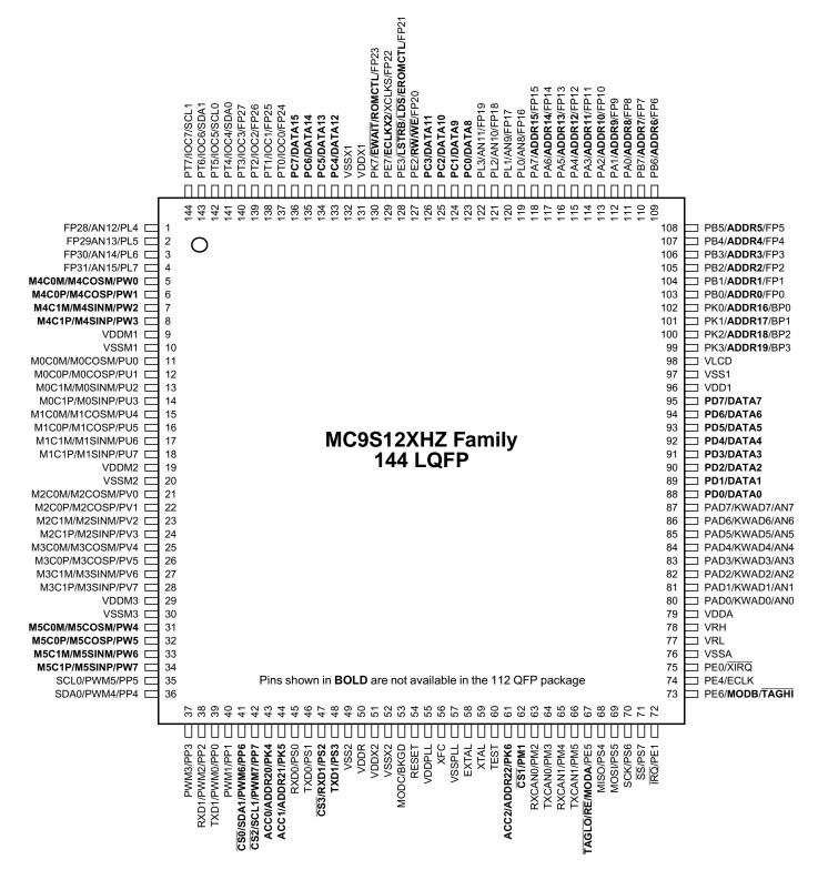
Figure 1-4. MC9S12XHZ Family 144 LQFP Pin Assignment
