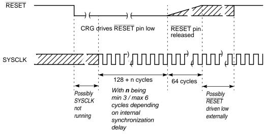
Figure 7-25. RESET Timing
