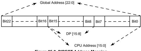
Figure 25-9. DIRECT Address Mapping
