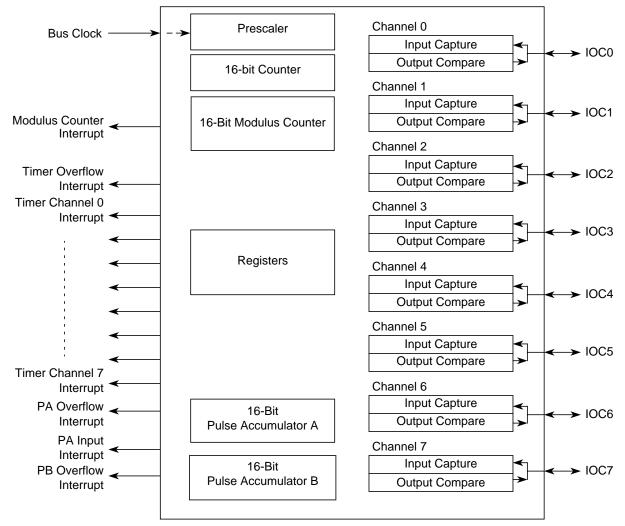
Figure 19-1. ECT Block Diagram
