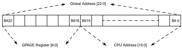
Figure 25-7. GPAGE Address Mapping
