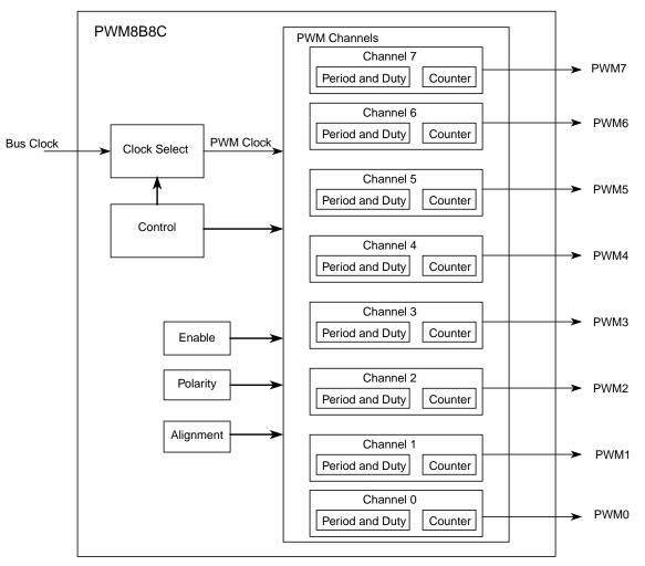
Figure 18-1. PWM Block Diagram
