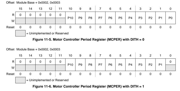
For example, programming MCPER to 0x0022 (PER = 34 decimal) will result in 34 counts for each complete PWM period. Setting MCPER to 0 will shut off all PWM channels as if MCAM[1:0] is set to 0 in all channel control registers after the next period timer counter overflow. In this case, the motor controller releases all pins.
