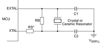
$^{\ast}$  Rs can be zero (shorted) when use with higher frequency crystals. Refer to manufacturer's data.
