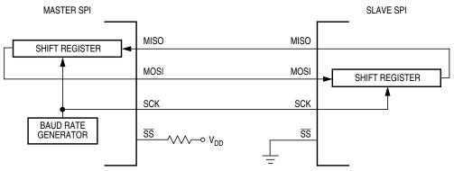
Figure 16-10. Master/Slave Transfer Block Diagram
