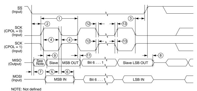
In Figure A-9 the timing diagram for slave mode with transmission format CPHA = 1 is depicted.
