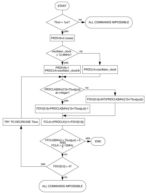
Figure 3-24. Determination Procedure for PRDIV8 and FDIV Bits
