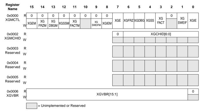
Figure 5-2. XGATE Register Summary (Sheet 1 of 3)
