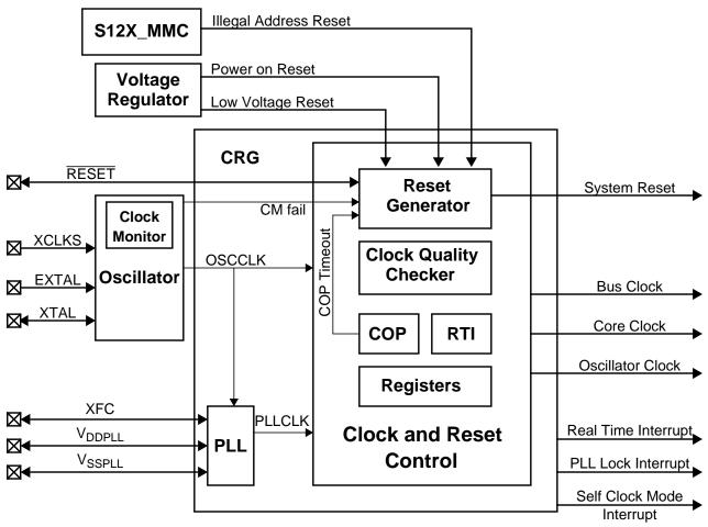
Figure 7-1. CRG Block Diagram
