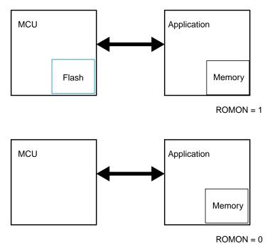
Figure 25-29. ROM in Normal Expanded Mode
