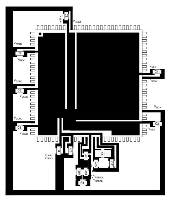
Figure C-2. LQFP112 Recommended PCB Layout
