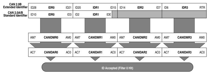
Figure 14-40. 32-bit Maskable Identifier Acceptance Filter
