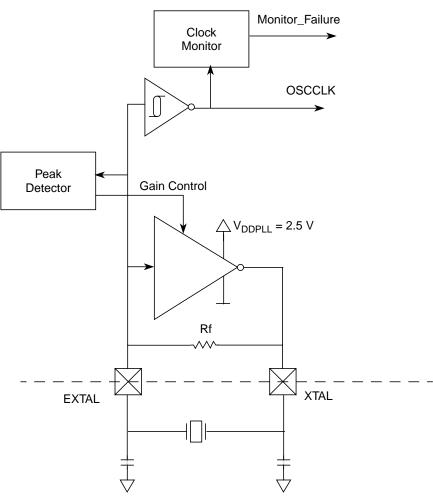
Figure 8-1. XOSC Block Diagram
