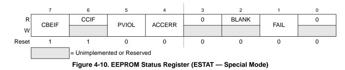
CBEIF, PVIOL, and ACCERR are readable and writable, CCIF and BLANK are readable and not writable, remaining bits read 0 and are not writable in normal mode. FAIL is readable and writable in special mode.
