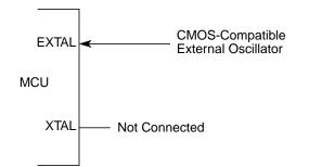
Figure 1-9. External Clock Connections (PE7 = 1)
