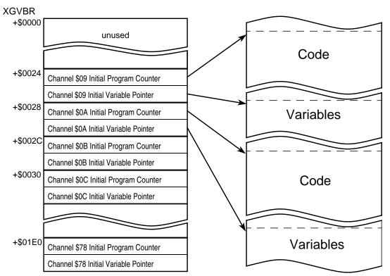
Figure 5-20. XGATE Vector Block
