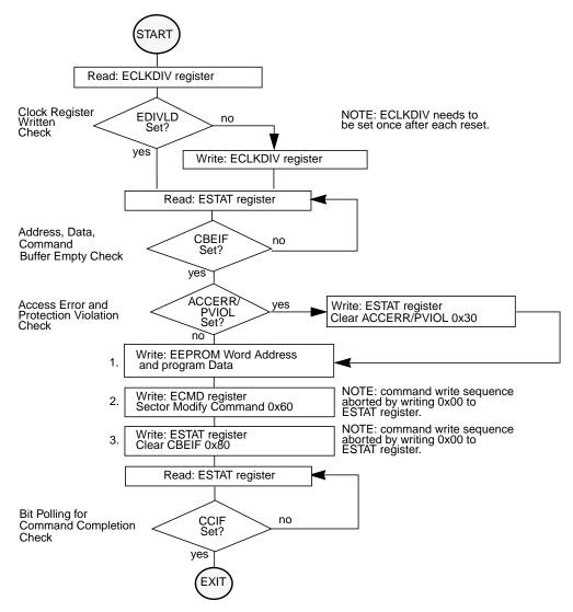
Figure 4-23. Example Sector Modify Command Flow
