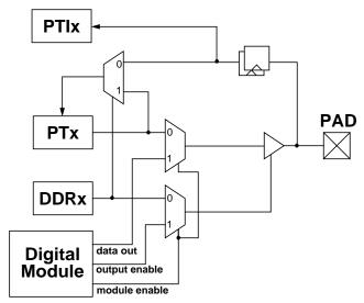
Figure 2-84. Illustration of I/O Pin Functionality
