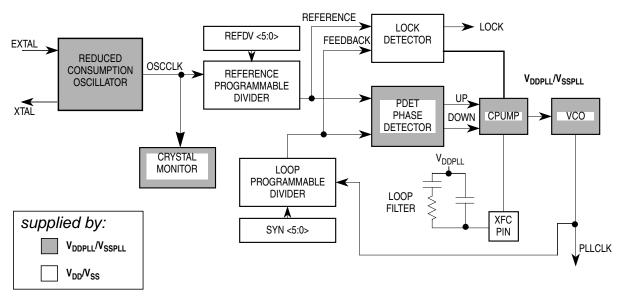
Figure 7-16. PLL Functional Diagram
