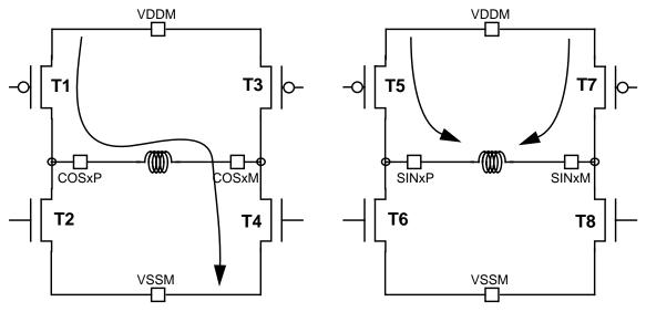
Figure 12-11. Current Flow when STEP = 0, DCOIL = 1, ITG = 0, RCIR = 0
