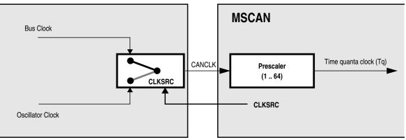
Figure 14-43. MSCAN Clocking Scheme
