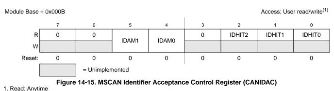
Write: Anytime in initialization mode (INITRQ = 1 and INITAK = 1), except bits IDHITx, which are read-only
