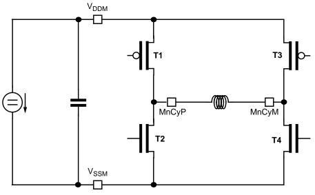
Figure 11-16. Output Transistor Assignment
