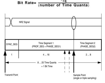
Figure 14-44. Segments within the Bit Time
