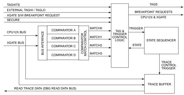
Figure 22-1. Debug Module Block Diagram
