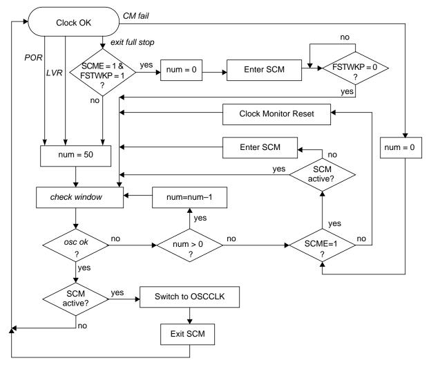
Figure 7-20. Sequence for Clock Quality Check
