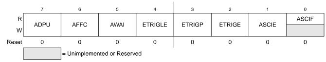
Figure 9-5. ATD Control Register 2 (ATDCTL2)
