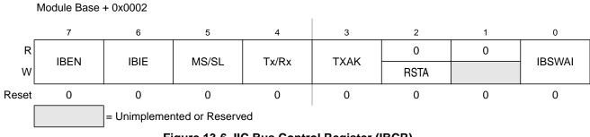
Figure 13-6. IIC Bus Control Register (IBCR)
