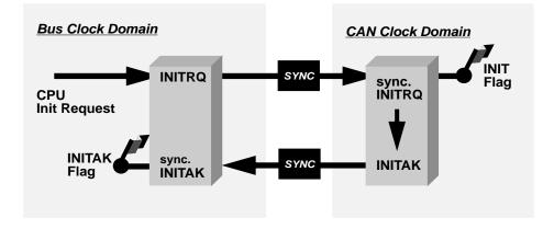
Figure 14-45. Initialization Request/Acknowledge Cycle
