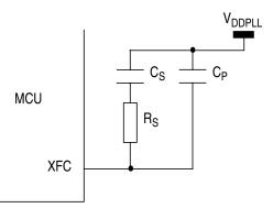
Figure 7-2. PLL Loop Filter Connections
