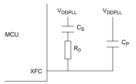
Figure 1-6. PLL Loop Filter Connections
