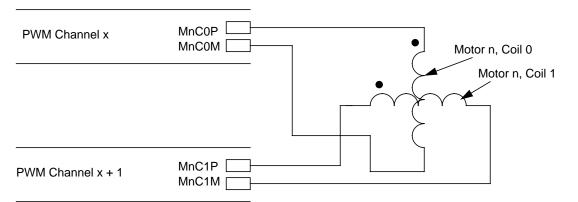
Figure 11-10. Typical Dual Full H-Bridge Mode Configuration
