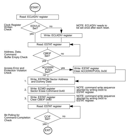
Figure 4-20. Example Sector Erase Command Flow
