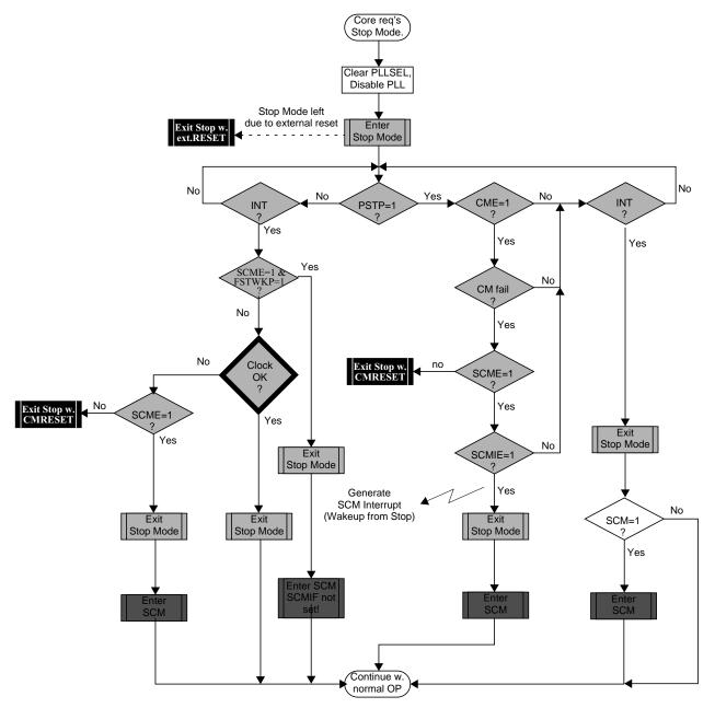
Figure 7-22. Stop Mode Entry/Exit Sequence
