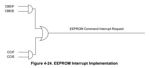
For a detailed description of the register bits, refer to Section 4.3.2.4, "EEPROM Configuration Register (ECNFG)" and Section 4.3.2.6, "EEPROM Status Register (ESTAT)".
