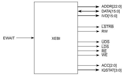
Figure 23-1. XEBI Block Diagram
