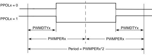
Figure 18-22. PWM Center Aligned Output Waveform
