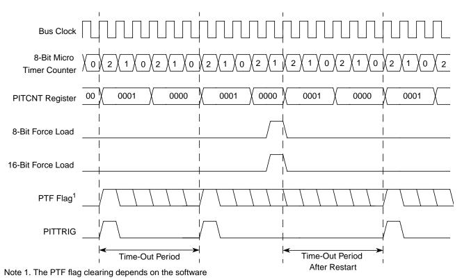
Figure 17-20. PIT Trigger and Flag Signal Timing
