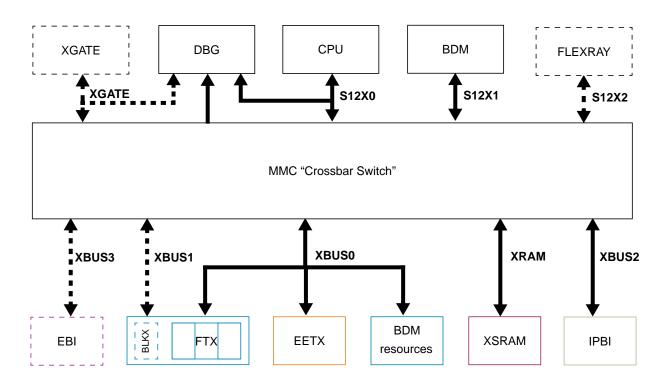
Figure 25-26. MMC Block Diagram
