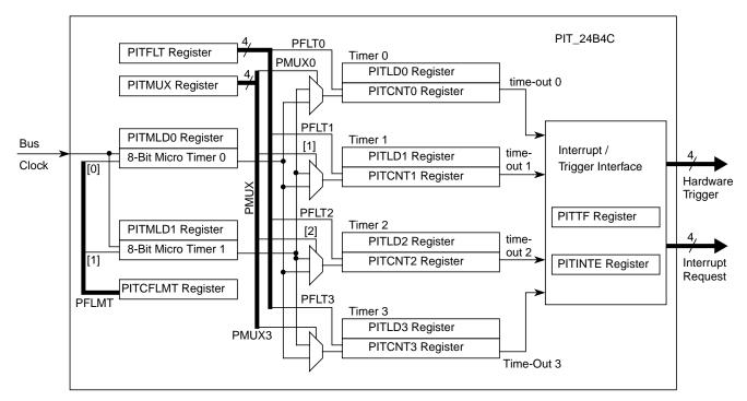
Figure 17-19. PIT Detailed Block Diagram
