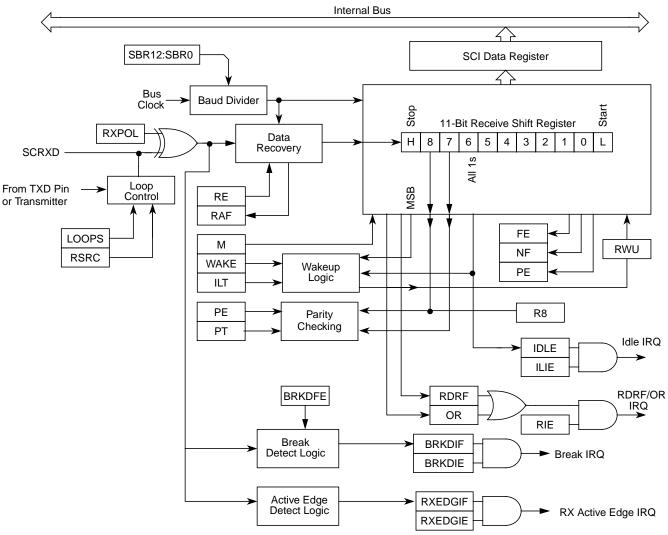
Figure 15-20. SCI Receiver Block Diagram
