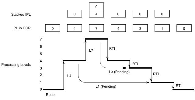
Figure 24-14. Interrupt Processing Example
