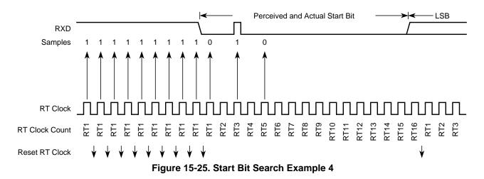
Figure 15-26 shows a burst of noise near the beginning of the start bit that resets the RT clock. The sample after the reset is low but is not preceded by three high samples that would qualify as a falling edge. Depending on the timing of the start bit search and on the data, the frame may be missed entirely or it may set the framing error flag.
