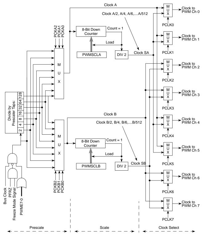
Figure 18-18. PWM Clock Select Block Diagram
