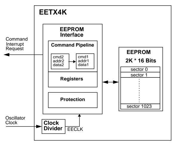
Figure 4-1. EETX4K Block Diagram
