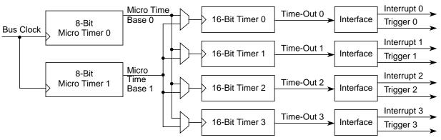
Figure 17-1. PIT Block Diagram
