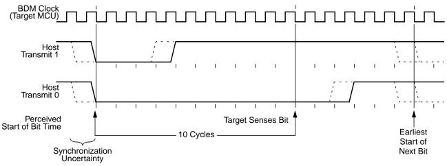
Figure 21-8. BDM Host-to-Target Serial Bit Timing
