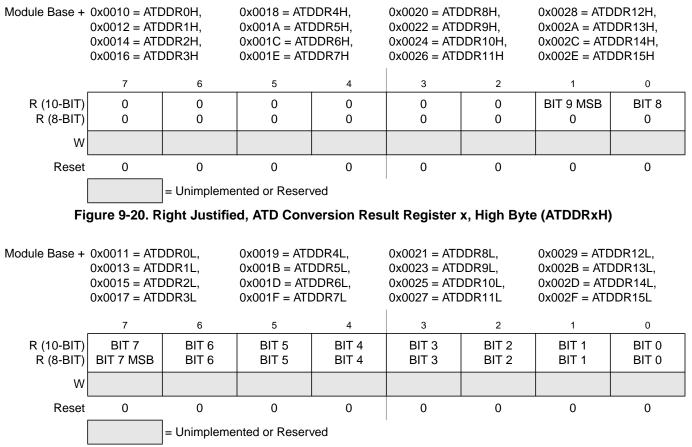
Figure 9-21. Right Justified, ATD Conversion Result Register x, Low Byte (ATDDRxL)
