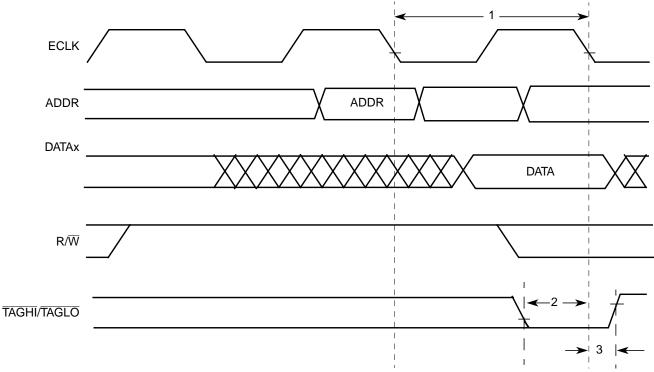
Figure A-16. External Trigger Timing
