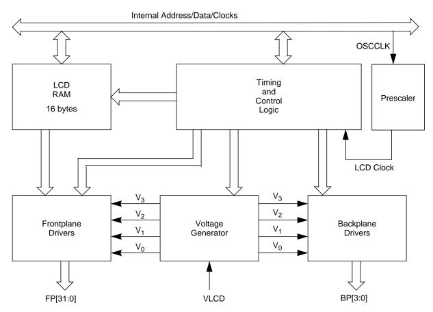
Figure 10-1. LCD32F4BV1 Block Diagram
