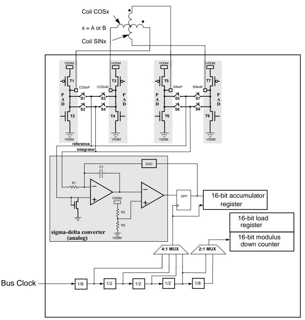
Figure 12-1. SSD Block Diagram
