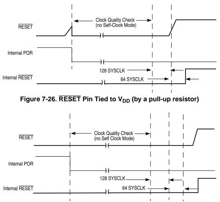
Figure 7-27. RESET Pin Held Low Externally
