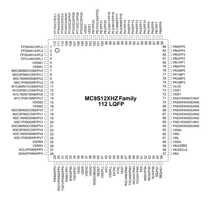
Figure 1-5. MC9S12XHZ Family 112 LQFP Pin Assignment
