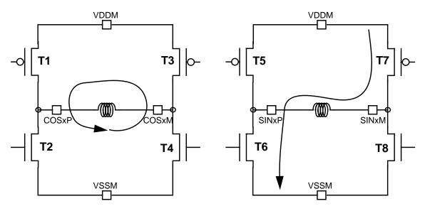
Figure 12-14. Current flow when STEP = 3, DCOIL = 1, ITG = 1
