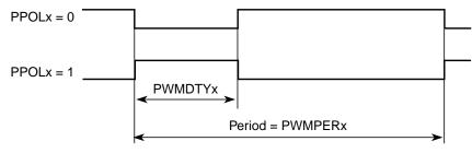
Figure 18-20. PWM Left Aligned Output Waveform
