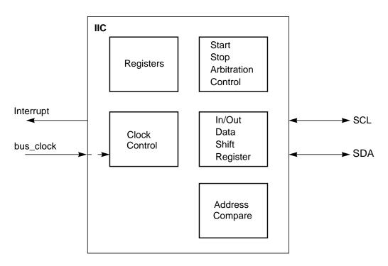
Figure 13-1. IIC Block Diagram
