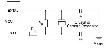
Figure 1-8. Full Swing Pierce Oscillator Connections (PE7 = 1)
