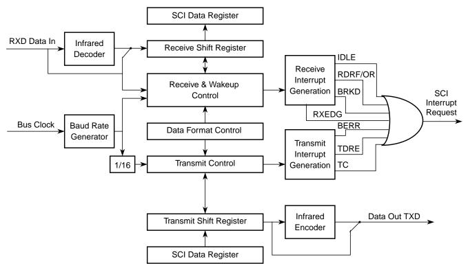
Figure 15-1. SCI Block Diagram
