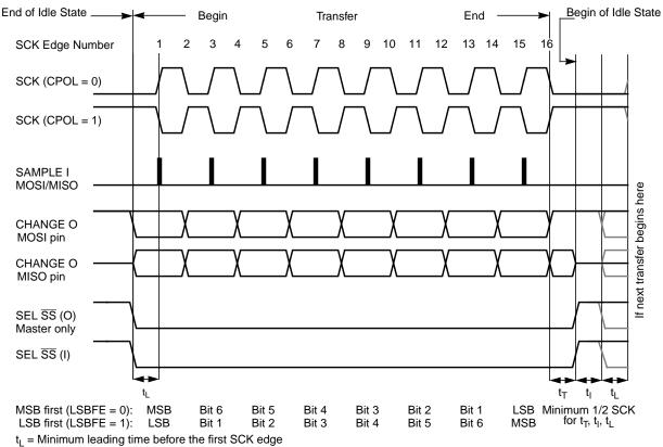
$t_{T}$  = Minimum trailing time after the last SCK edge
