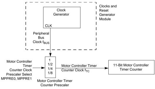
Figure 11-22. Motor Controller Counter Clock Selection
