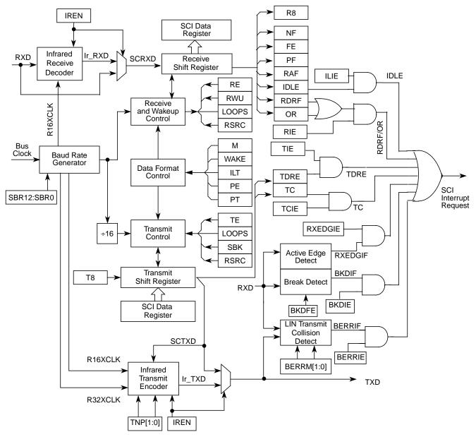
Figure 15-14. Detailed SCI Block Diagram
