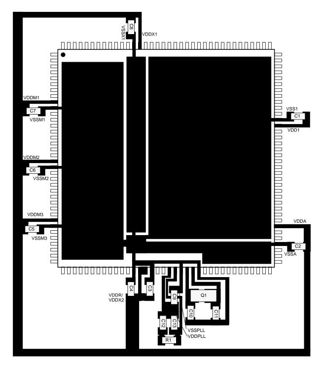
Figure C-1. LQFP144 Recommended PCB Layout
