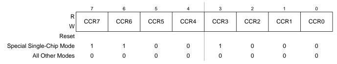
Figure 21-4. BDM CCR LOW Holding Register (BDMCCRL)
