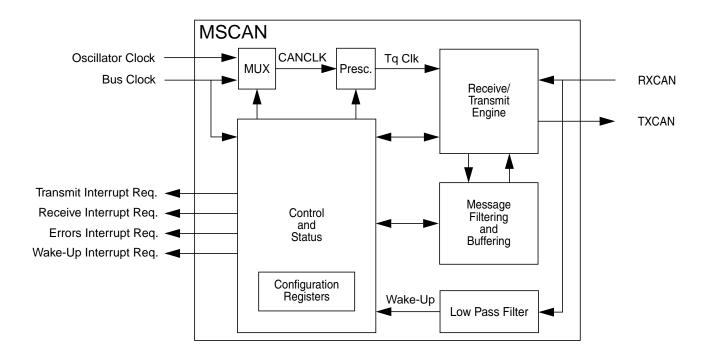
Figure 14-1. MSCAN Block Diagram
