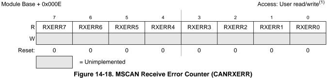
1. Read: Only when in sleep mode (SLPRQ = 1 and SLPAK = 1) or initialization mode (INITRQ = 1 and INITAK = 1) Write: Unimplemented
