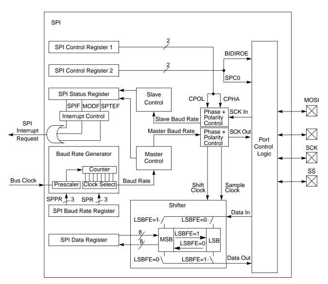
Figure 16-1. SPI Block Diagram
