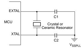
Figure 8-2. Loop Controlled Pierce Oscillator Connections (XCLKS = 0)
