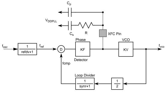
Figure A-3. Basic PLL Functional Diagram
