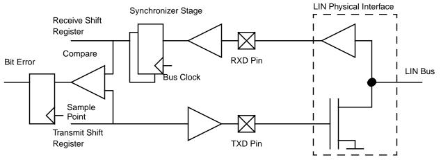
Figure 15-18. Collision Detect Principle
