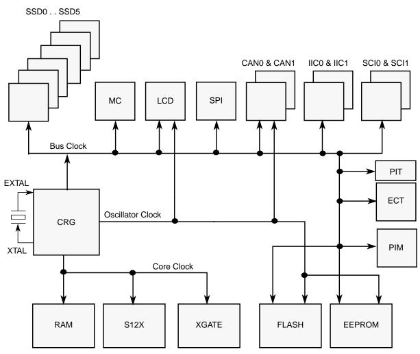
Figure 1-10. Clock Connections
