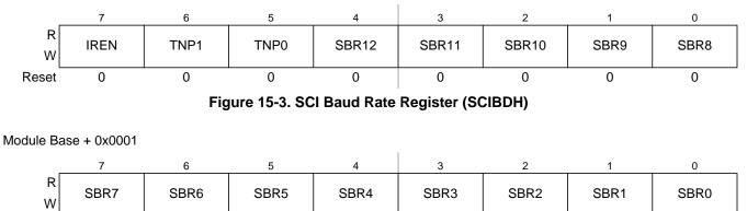
Figure 15-4. SCI Baud Rate Register (SCIBDL)
