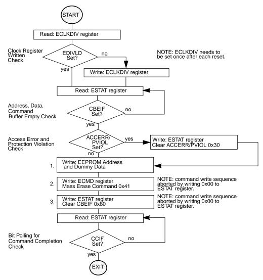
Figure 4-21. Example Mass Erase Command Flow
