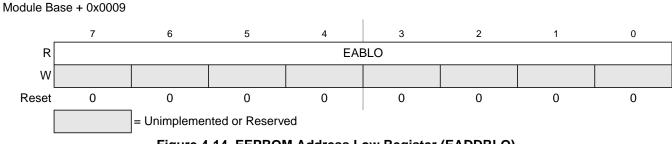
Figure 4-14. EEPROM Address Low Register (EADDRLO)
