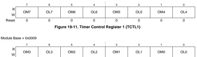
Figure 19-12. Timer Control Register 2 (TCTL2)
