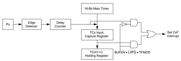
Figure 19-73. Block Diagram for Port 7 with Output Compare/Pulse Accumulator A
