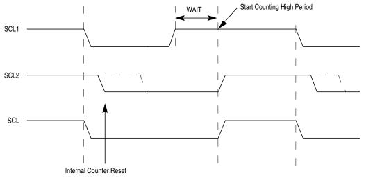
Figure 13-12. IIC-Bus Clock Synchronization
