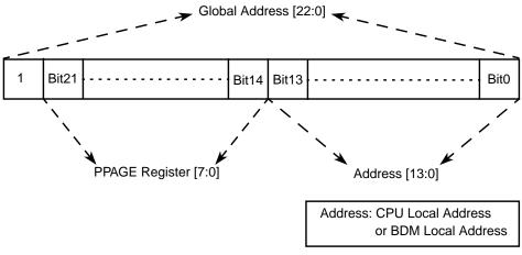
Figure 25-16. PPAGE Address Mapping
