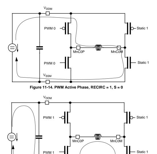
Figure 11-15. PWM Passive Phase, RECIRC = 1, S = 0
