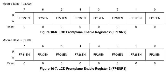
These bits enable the frontplane output waveform on the corresponding frontplane pin when LCDEN = 1.
