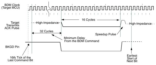
Figure 21-11. Target Acknowledge Pulse (ACK)
