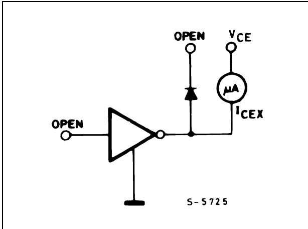
Figure 4. Output leakage current (for ULN2002 only)
