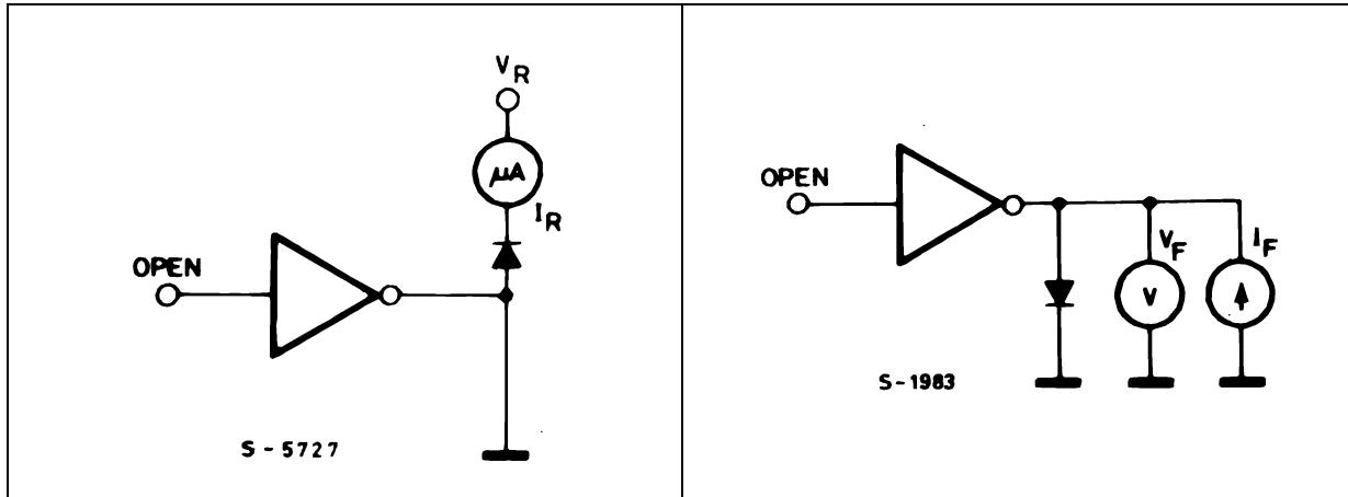
**Figure 10. Clamp diode forward voltage**
