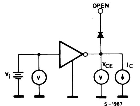
**Figure 9. Clamp diode leakage current**
