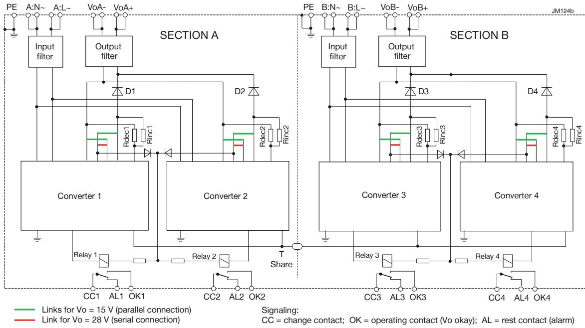
Fig. 2a - Single output system
