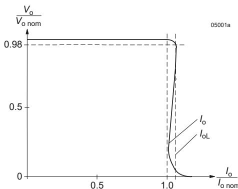
Fig. 7. Typical output characteristic  $V_o$  versus  $I_o$ .
