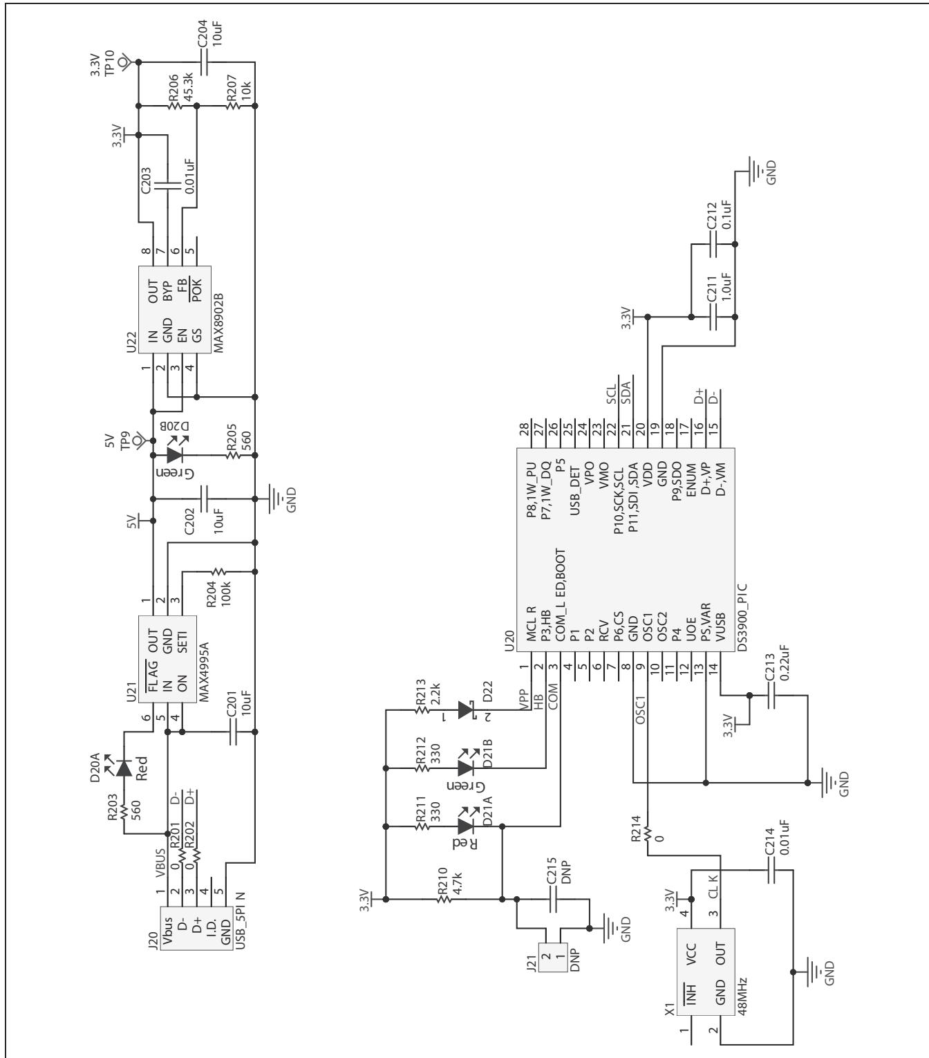
Figure 2b. DS4404 EV Kit Schematic (Sheet 2 of 2)
