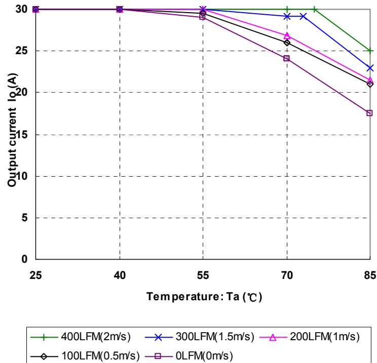
Figure 17 Output power derating, 48V<sub>in</sub>, air flowing across the converter from V<sub>in-</sub> and V<sub>in+</sub>
