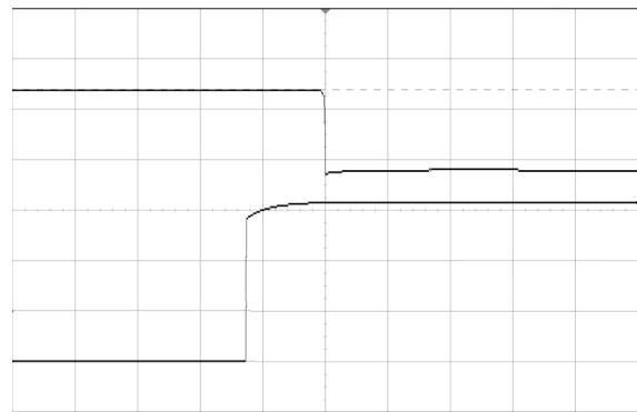
Figure 9 Output voltage shutdown by remote OFF,
