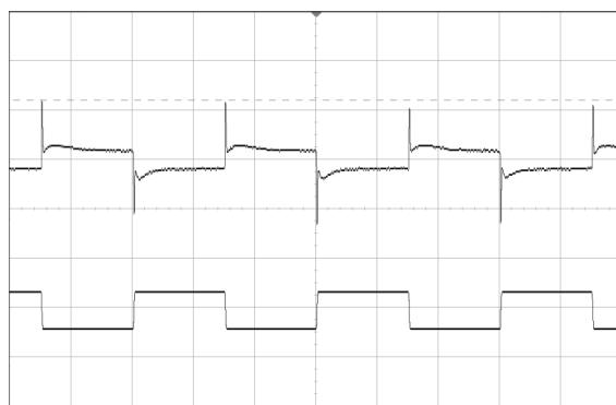
Figure 4 Dynamic response for 25% load step (25% ~ 50% ~ 25%) and 0.1A/μs slew rate, (2ms/div), see Figure 10 for test configuration; CH1-output voltage (50mV/div); CH2-output current (10A/div)
