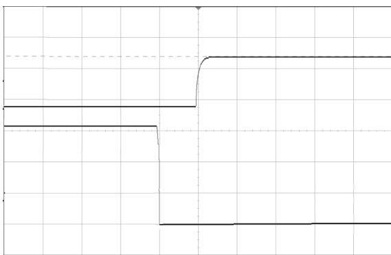
Figure 8 Output voltage startup by remote ON,
