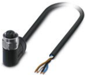
Sensor/Actuator cable, 4-position, PE-X halogen-free, black-gray RAL 7021, free cable end, on Socket angled M12, A-coded, Cable length: 2 m, for outdoor applications, with high-grade steel knurl
