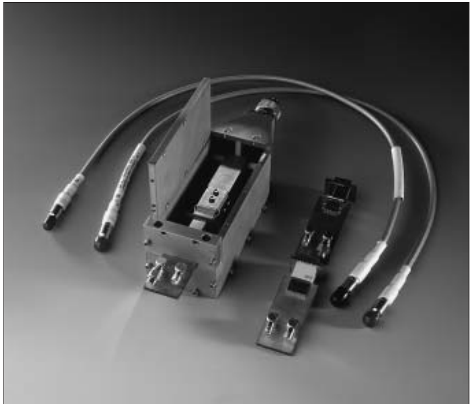
Fig.7 : Triaxial test cel
