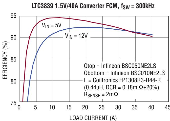
Figure 2. Efficiency Curves for the DC1632A in FCM
