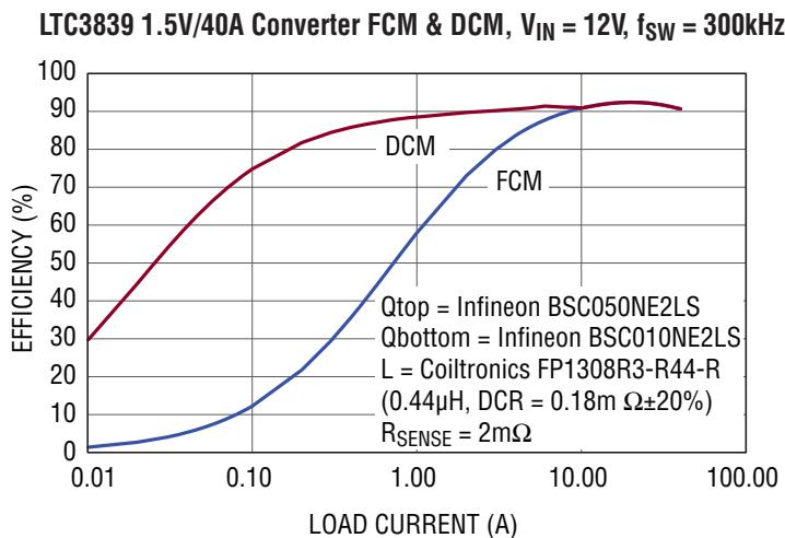
Figure 3. Efficiency Curves for the DC1632A in FCM and DCM
