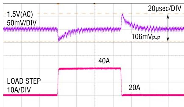
Figure 4. Load Step Response of the DC1632A at  $V_{IN} = 12V$ .  $C_{OUT} = 4 \times$  Sanyo 2R5TPE330M9 ||  $2 \times 100\mu\text{F}$  X5R 6.3V 1206,  $L_1, 2 = 0.44\mu\text{H}$ ,  $f_{SW}=300\text{kHz}$
