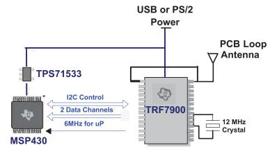
The TRF7900 simplifies system design by reducing system component count and manual circuit tuning. By integrating the PLL, SAW filter, and RF mixer, the TRF7900 eliminates the manual tuning of RLC circuits required in traditional implementations.
