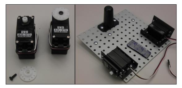
7. Take out the two wheels and the rubber traction bands. Stretch the rubber band around the outside of the wheel. Then, attach the wheels to the servos, and secure them using the small black screws that were removed in the previous step.
