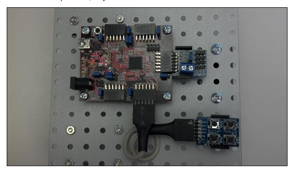
10. Connect the right servo to J4 and the left servo to J5 on the PmodCON3. The white cable must be connected to the pin labeled "SIG".
