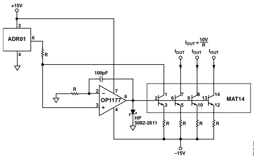
Figure 18. Temperature Independent Current Sink,  $I_{OUT} = 10\text{ V/R}$
