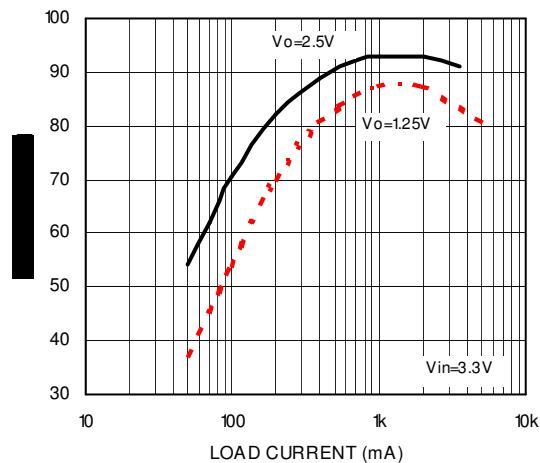
Figure 3. Efficiency vs load current (550KHz)
