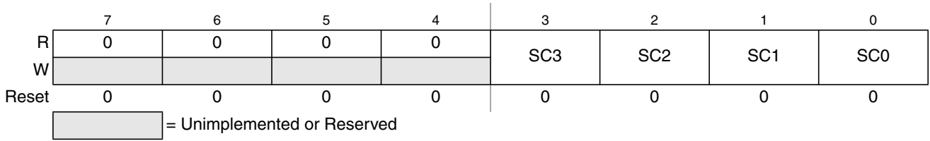
Figure 6-11. Debug State Control Register 3 (DBGSCR3)
