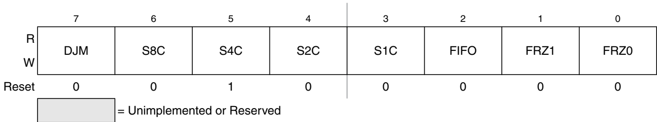
Figure 8-6. ATD Control Register 3 (ATDCTL3)
